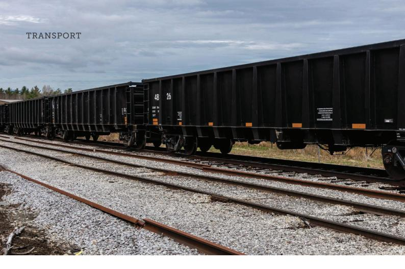
A 65-foot gondola, coated in black acrylic, can carry cargos that are impervious to weather conditions, including metal, coal, coke, aggregates, sand, ores, gravel, slag, scrap, poles, railroad ties and other goods. making them a viable alternative for epoxies. As the rail industry continues to compete with truck-based shipping, rail owners and operators must find ways to ensure the industry remains the lowest cost mode of transporting freight – and water-based acrylics are playing a key role.
