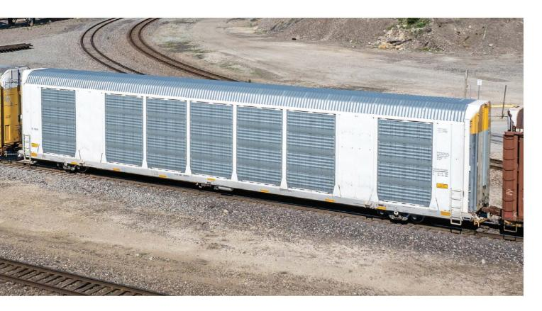
Ensuring that all surfaces of autoracks are fully coated is critical, as any exposed steel surfaces can cause rust bleeding which could damage exterior paint of new automobiles.
