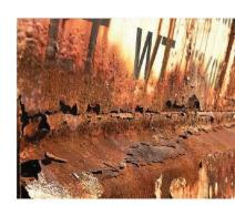
FIG. 1: The exterior of this hopper car is protected by a single coat of direct-to-metal (DTM) epoxy. This widespread corrosion is typical of rail cars in salt service.
