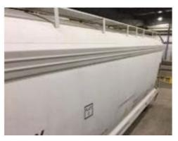
FIG. 2: The corrosion protection package for this hopper car in salt service consisted of a zinc-rich primer followed by an epoxy. The photograph was taken five years after system installation.
