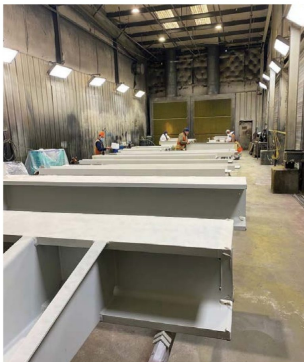
FIG. 4: Off-site application shops feature wide-open settings and sufficient space to access steel for better fireproofing applications and easier inspections.
