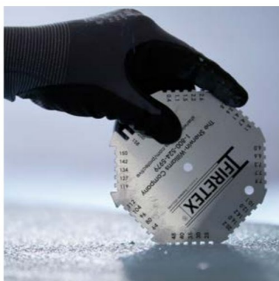
FIG. 5: Checking the wet film thickness (WFT) of fireproofing coatings is much easier when working on the ground in a shop environment compared to taking measurements while on lifts, scaffolding or ladders in the field.
