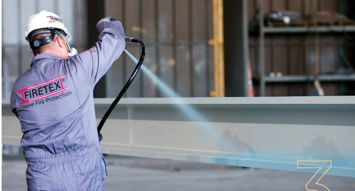
FIG. 6: For in-shop applications, applicators can easily position themselves for better spray control and a more consistent film build.
