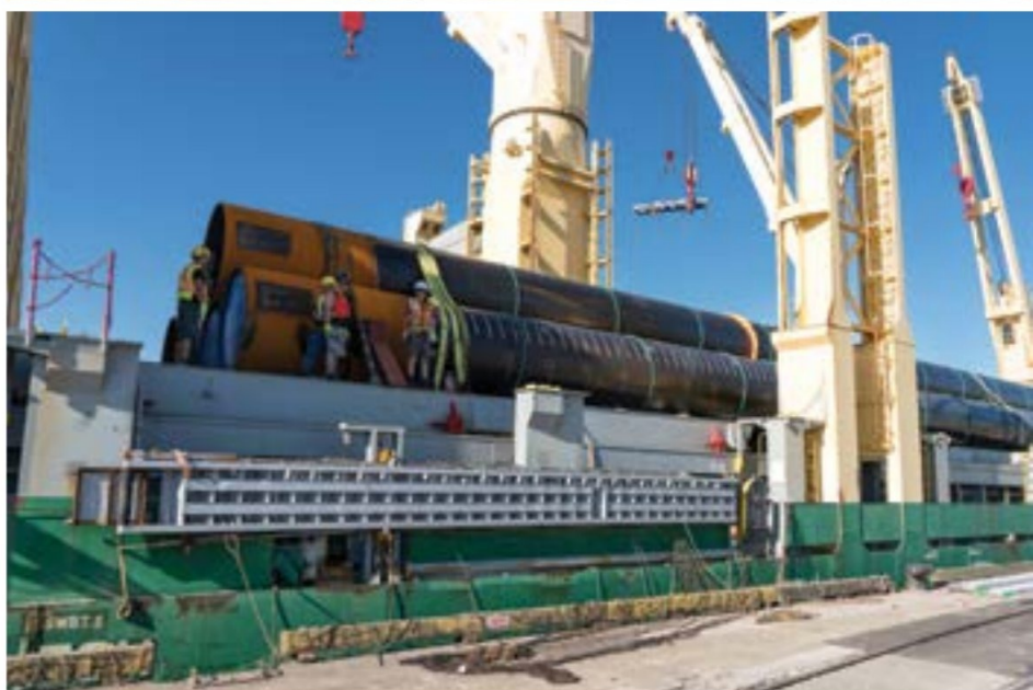
FIG. 5: Steel pilings coated externally with Hydrocarbon-Modified Epoxy Coating A.
