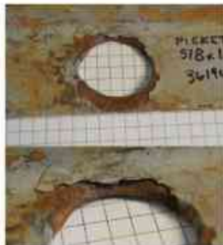
Fig. 8: Slotted bolt hole in Sample 2. The bottom image shows the smooth attack in the width of the slot. There is cracking of the coating and the attack is undercut beneath the coating. The red outline in the top image shows approximate original dimensions of the bolt hole.
