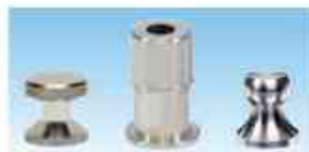
Fig. 3: Dollies for Type II (fixed alignment), Type III and Type V (self-aligning) pull-off testers
