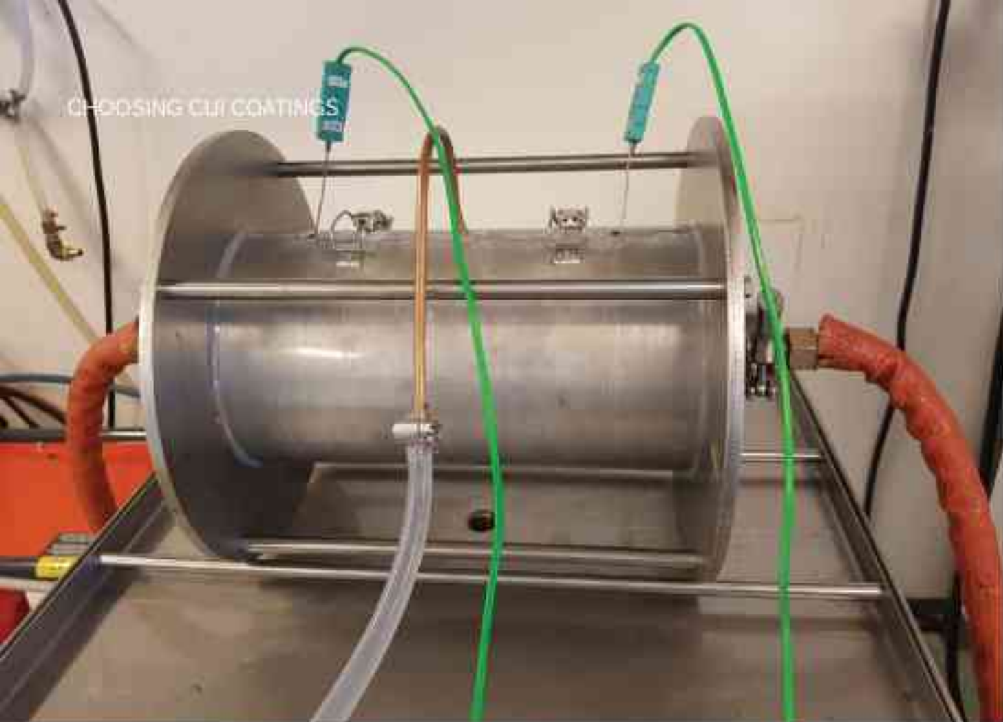
Fig. 3: A small-scale test rig adapted from ASTM G-189.
