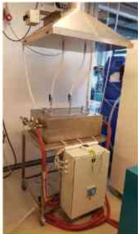
Fig. 4: Equipment used for multi-phase CUI cyclic corrosion testing.
