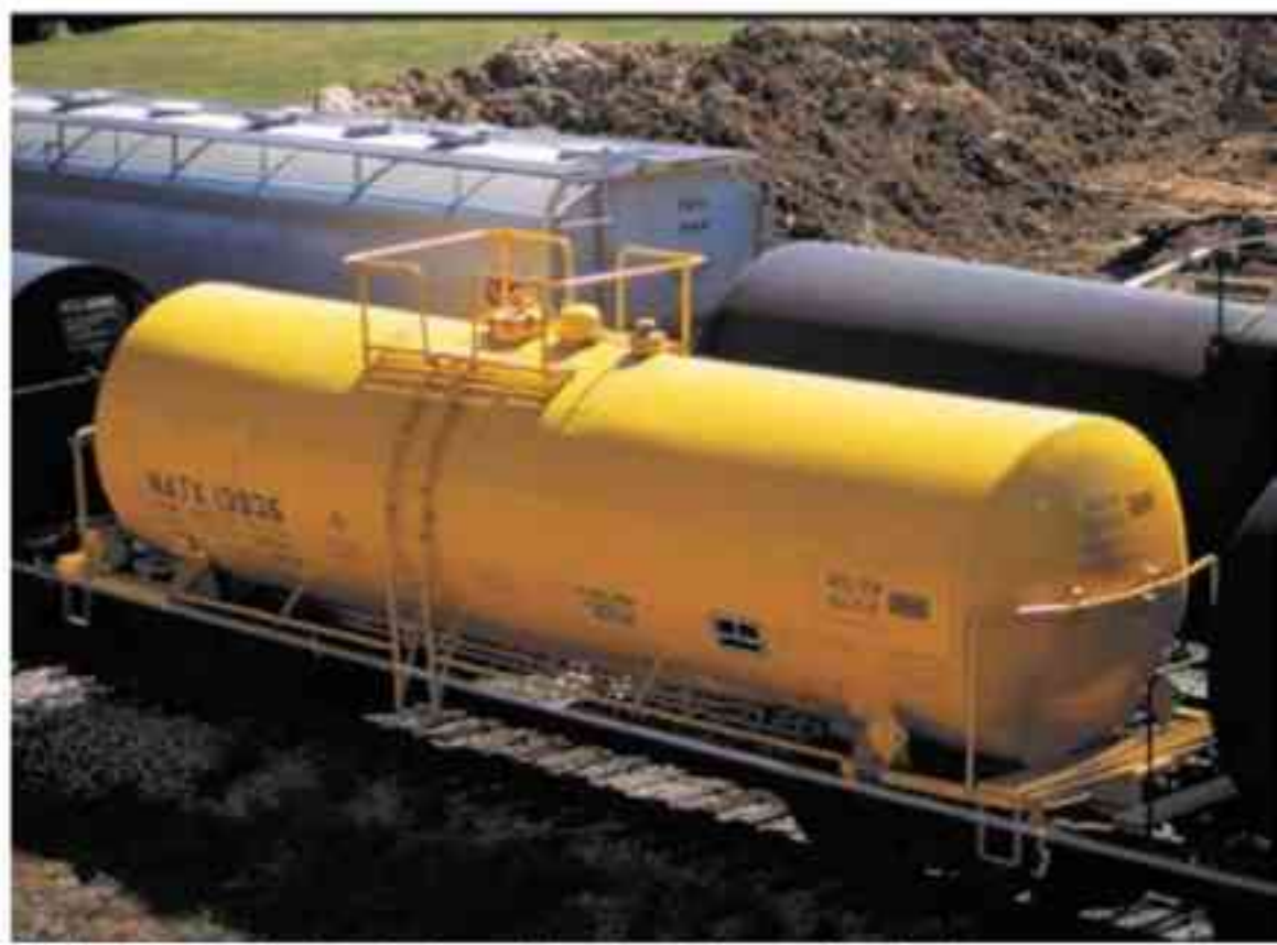
Fig. 1 Most freight cars, such as the tank and pressure-differential covered hopper cars shown here, feature one-coat, direct-to-metal (DTM) epoxy coatings. Photos courtesy of The Sherwin-Williams Company unless otherwise noted.
