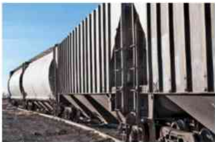
Fig. 3: While epoxy coatings will chalk and change color over time—as shown on these freight railcars—such changes do not affect the coating's corrosion resistance.
