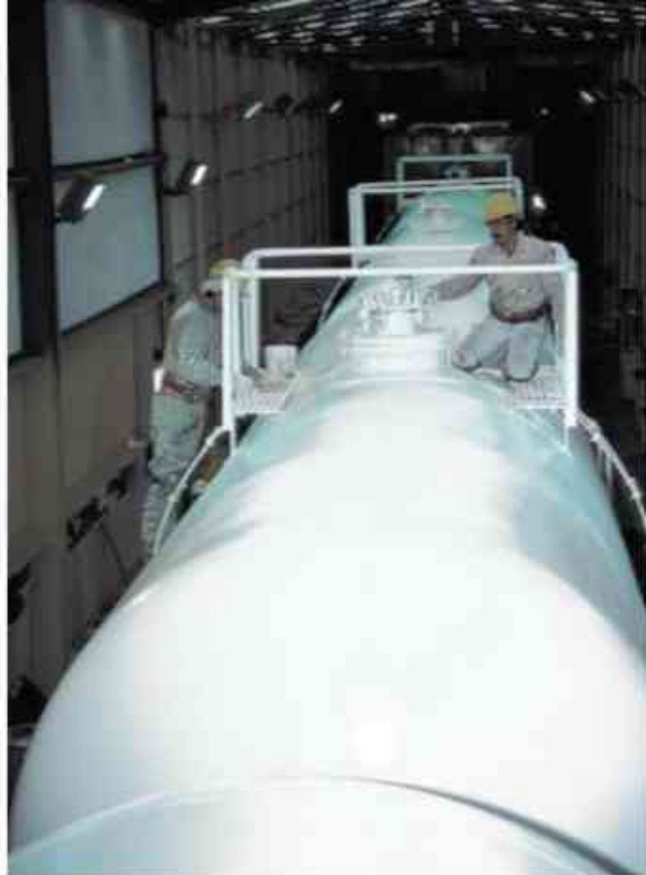
Fig. 3: Applicators inspect the final finish of a tank car before moving the car out of the paint shop for stenciling.
