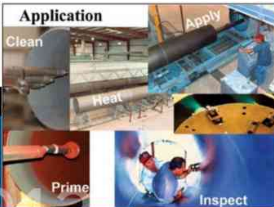
Application of internal linings is straightforward: clean, heat, prime (if necessary), apply FBE, cure, cool and inspect. Photos courtesy of Alan Kehr.
