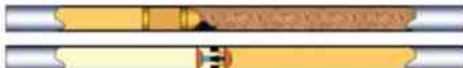
Mechanical scraping (top) and brush cleaning. Figures courtesy of MOGSIL.
