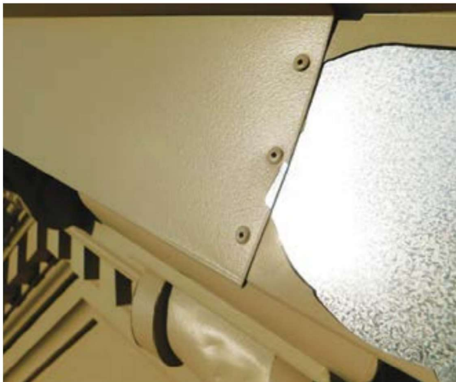
Fig. 1: Location of the coating failures on thin-gauge metal. Note that the delamination initiated at an edge of the galvanized steel. Figures courtesy of KTA-Tator, Inc.
