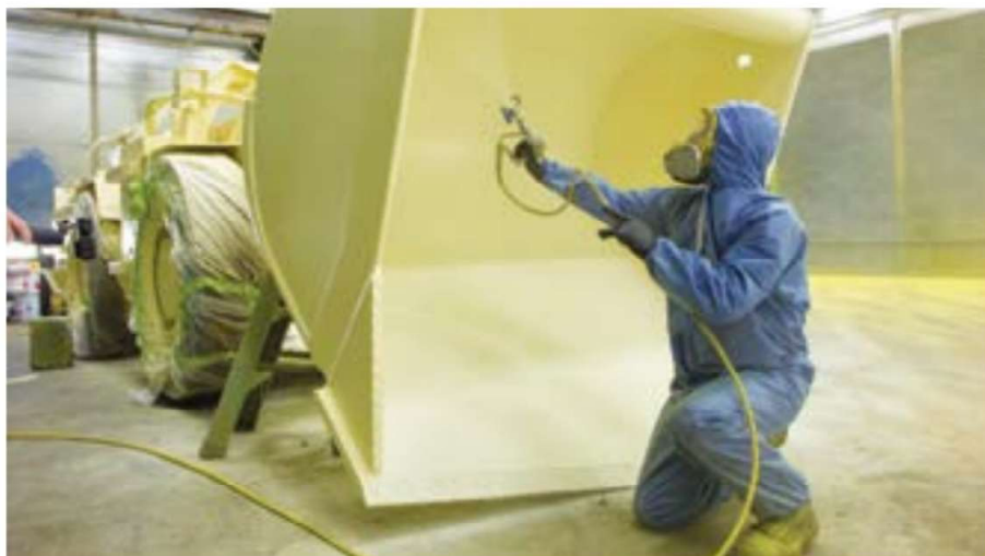
Fig. 3: The key to airless spraying is providing enough fluid pressure at the gun to atomize the material into a pattern that provides consistent coverage.
