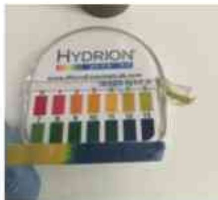
Fig. 3: Measurement of a solution using pH indicating paper.
