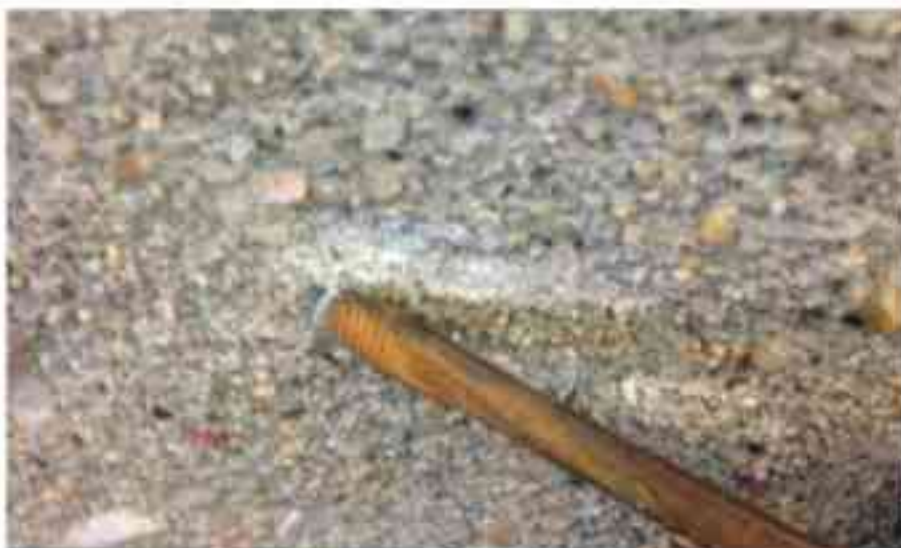
Fig. 2: Removing approximately 1 mm of cement paste
