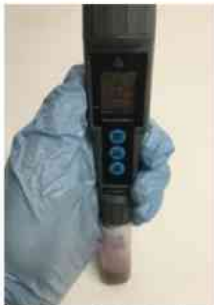
Fig. 5: Measurement of a solution using a pH meter.
