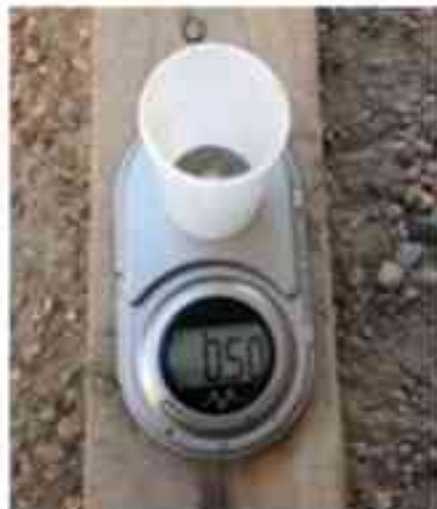
Fig. 4: Weighing concrete paste using a digital gram scale.
