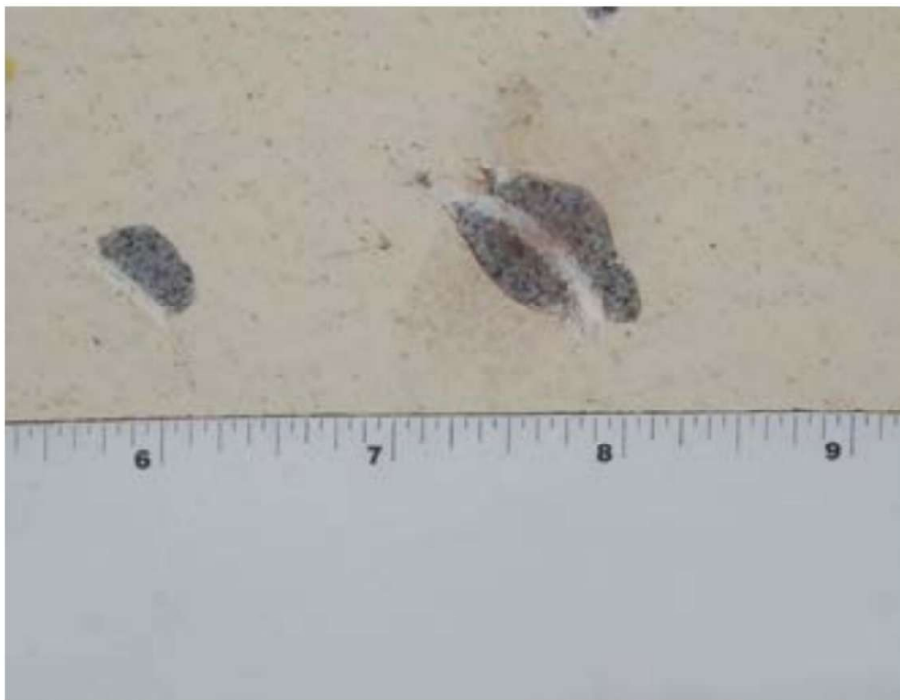
Fig. 4: Mechanical damage of the lining.
