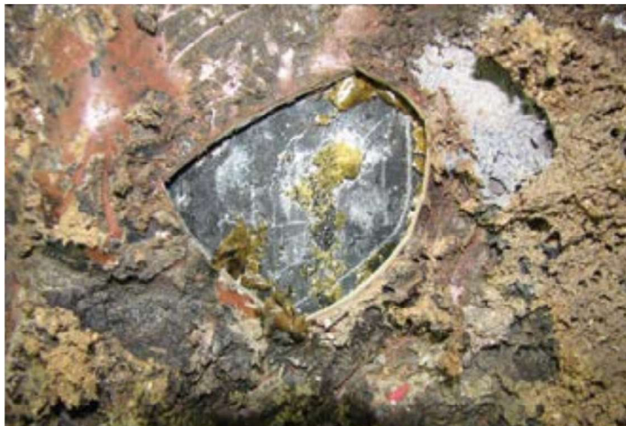
Fig. 6: At the waterline, delamination and primer degradation occurred.
