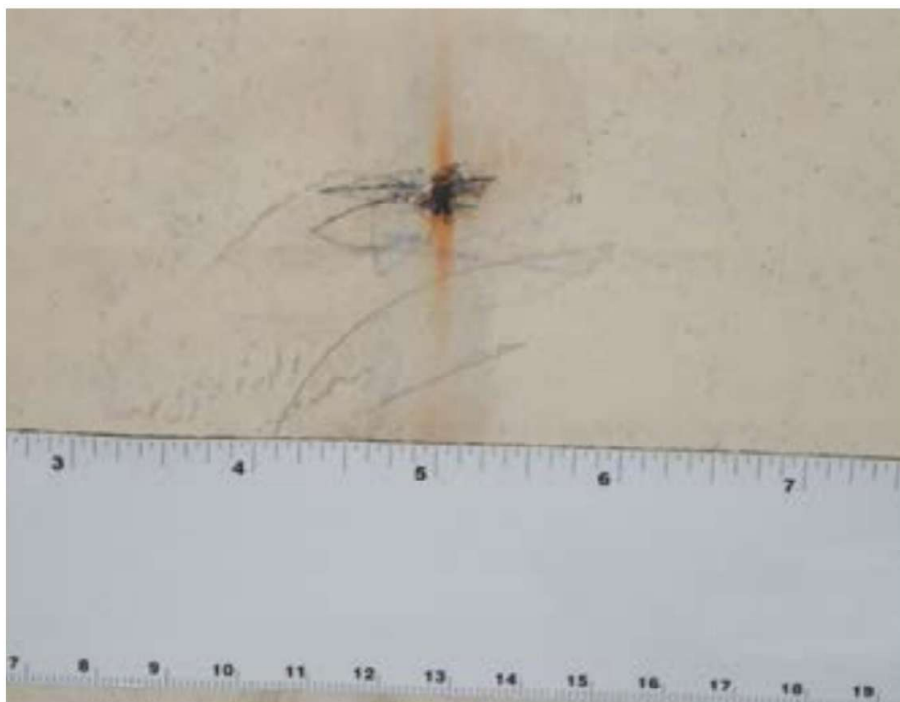
Fig. 3: View of spot corrosion above the waterline.
