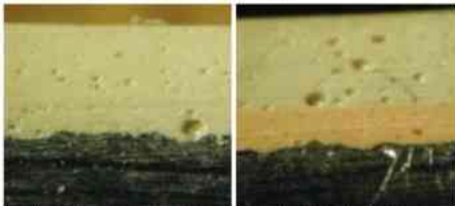
Fig. 8: Lining systems cross section. Holding primer/SFE: good wetting by the solvent-borne epoxy holding primer (left) and SFE: good wetting by the SFE (right).
