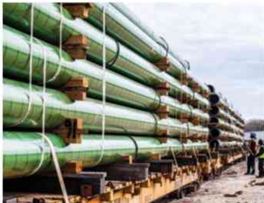
Fig. 4: A preventive anticorrosion FBE layer applied to pipes should offer good adhesion and resistance to cracking, cold flow and softening over a broad temperature range.
