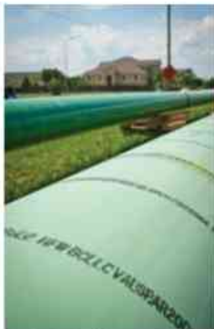
Fig. 2: Non-shielding FBE barrier coatings permit some electrical conductivity to the metal pipe so backup ICCP systems can maintain protection in areas of cathodic disbondment.
