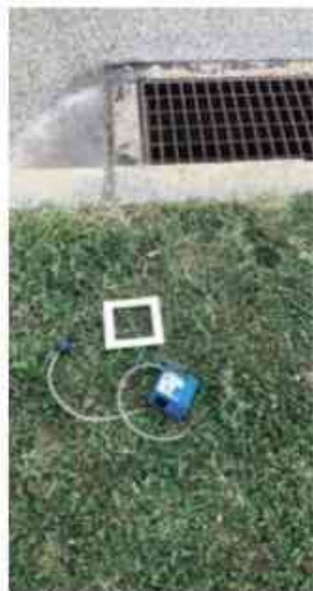
Fig. 2: In accordance with ASTM D7144, "Standard Practice for Collection of Surface Dust by Micro-Vacuum Sampling for Subsequent Metals Determination" the author collected a sample of visible debris observed near a storm drain.
