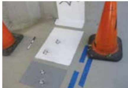
Fig. 4: Dollies adhered to various materials in anticipation of pull-off tests. Duct tape was used to secure dollies in place on vertical surfaces until the adhesive cured.
