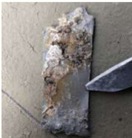
Fig. 1: The back side of the coating exhibited surface crazing. The surface crack did not penetrate the coating film, thus confirming that the distress is crazing. Photos courtesy of the author.
