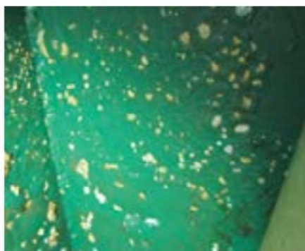
Fig. 4: Numerous blisters in the corner of one particular tank.
