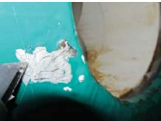
Fig. 3: White corrosion product underneath blisters in the lining that was removed.
