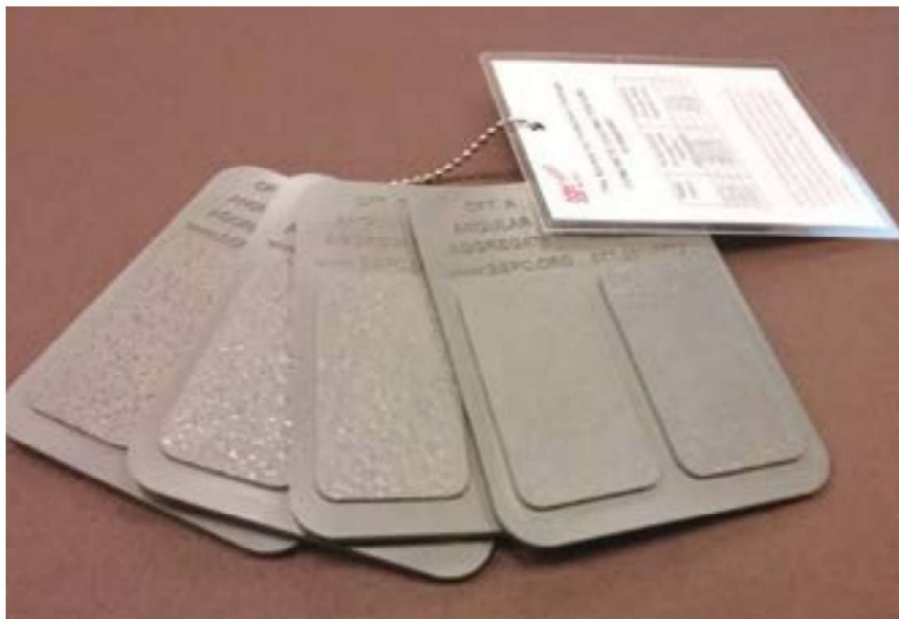
Fig. 2: Tactile texture comparator sets have been produced to provide a simple and efficient means of selecting, communicating and comparing the desired texture for an application. Photo courtesy of SSPC.
