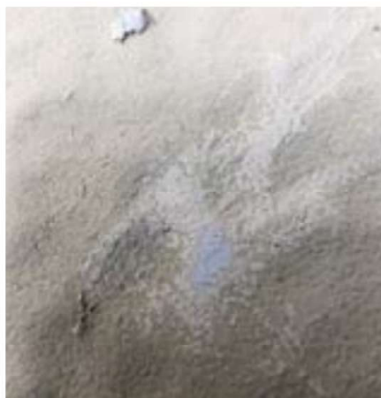
Fig. 2: Scraping away the top oxidized layer, exposing the pristine coating underneath.
