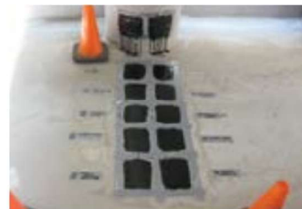
Fig. 3: Mock-up of test materials applied to vertical and horizontal surfaces. The grid represents different levels of surface preparation and in this case, the use of a primer (left) and without primer (right).
