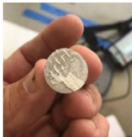
Fig. 5: One of dozens of pull-off tests indicating a “good pull.” This dolly shows cohesive failure of the coating system—ironically a good result indicating that the failure occurred within the coating film, as well as adhesive failure—also a good result indicating that the coating was so strongly adhered to the substrate that the glue holding the dolly failed before the coating pulled away from the substrate.
