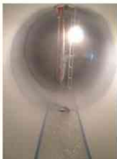
Fig. 1: A baked phenolic lining applied to the interior of a phenol-carrying tank car has protected the underlying substrate from both corrosion and chemical attack for 24 years, passing two different inspection cycles. Photos courtesy of Carboline Company.
