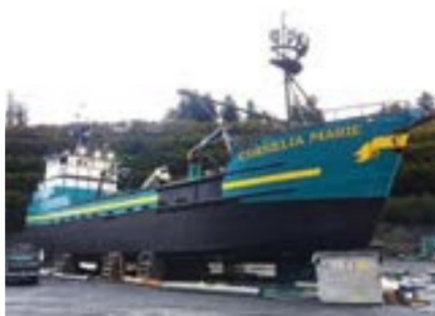
Fig. 7: Work on the underwater hull and freeboard of the Cornelia Marie involved taking the surfaces down to an existing tight antifouling coat, priming exposed bare steel, edge feathering above the waterline and spray-applying primer, an antifouling epoxy and an acrylic polyurethane gloss coating.
