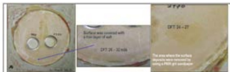
Fig. 3: Color, DFT and adhesion on Sample 2.
