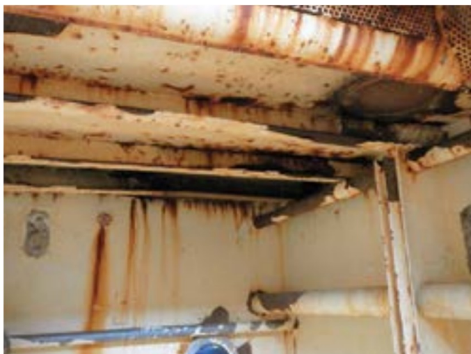
Figs. 1 and 2: The Cornelia Marie 's six fish holds showed visible signs of corrosion.
