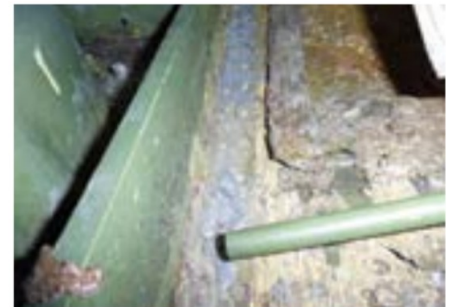
Fig. 2: HC-130 corrosion at Patrick Air Force Base.
