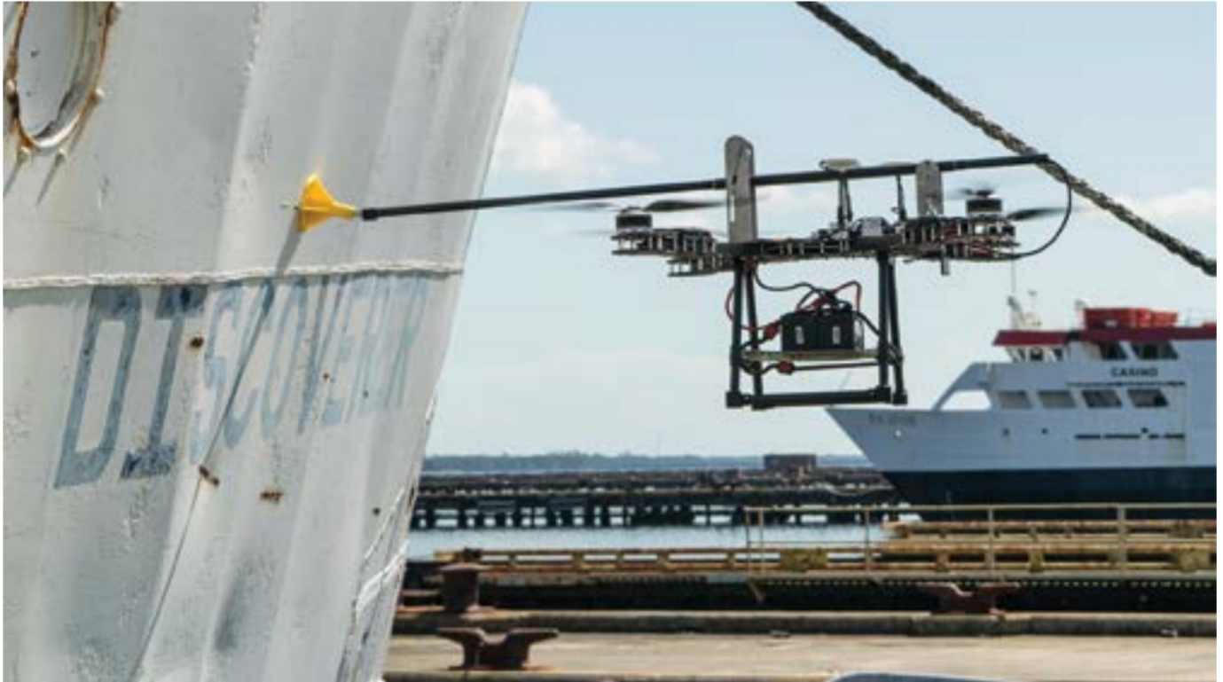
Fig. 1: Robotic aircraft takes DFT readings on a ship. Photo courtesy of Jeremy Countryman.
