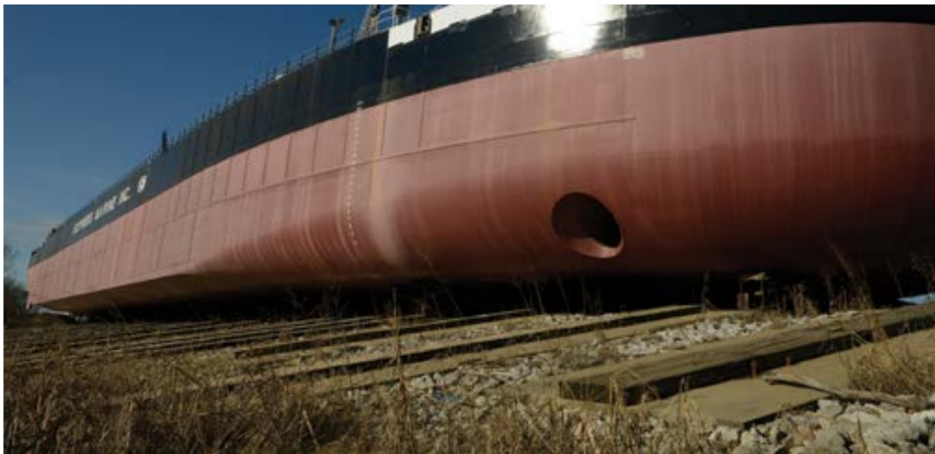
Exterior above-waterline surfaces received a polysiloxane finish coat for UV resistance and longevity.
