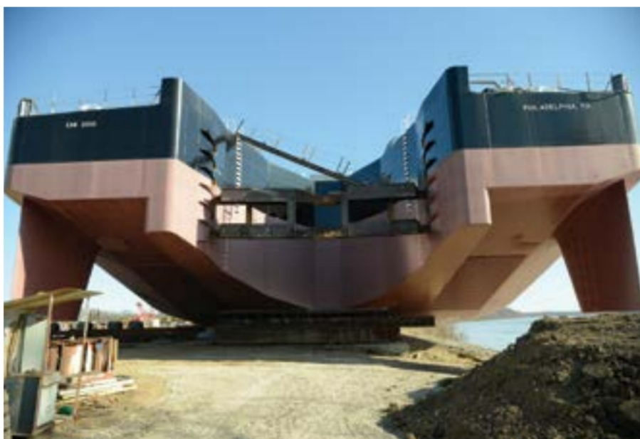
A number of coating systems were utilized on the new barge, including dual stripe and finish coats on difficult-to-access ballast tank edges and an abrasion-resistant epoxy for cargo hold areas.
