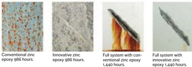
Fig. 1: Coating comparison after salt-spray testing. Figures courtesy of the author unless otherwise noted.
