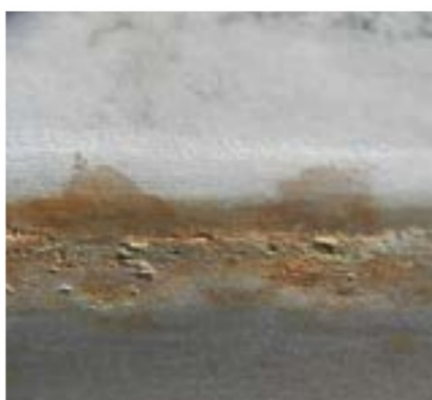
Fig. 8: Chlorides concentrate on stainless steel surfaces, especially at the water line and where metal surfaces are hot from direct sunlight exposure.
