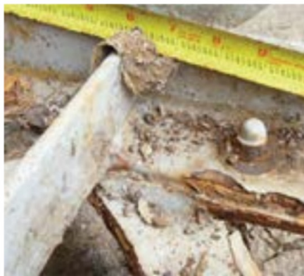
Fig. 1: Pitting at breaches in the coating typically has relatively high corrosion rates due to the large cathodic (coated steel) area relative to the very small anodic (coating failure or lack of coating) area as shown. All figures courtesy of the author unless otherwise noted.
