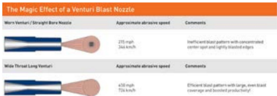
Fig. 3: A Venturi-style abrasive blasting nozzle works like a jet engine. Air is compressed rapidly in a cone, then passes through a small orifice and then expands at a more gradual rate than it compressed.
