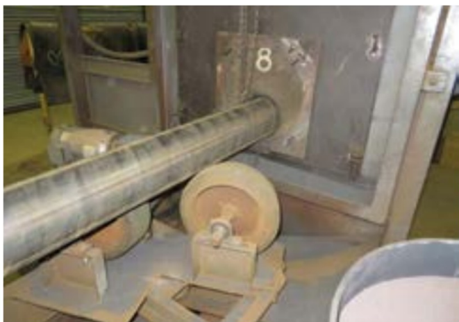
Fig. 5: Pipe entering shot-blasting machine.
