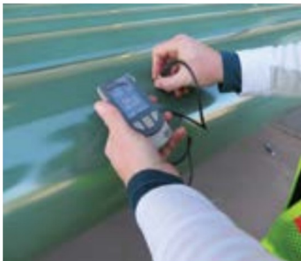
Fig. 11: Taking dry-film-thickness measurements.
