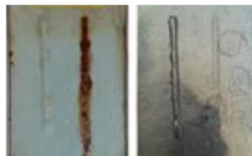
Fig. 6: System 1 edge-retentive epoxy 15-mil-thick coating at the end of exposure (left) and after coating removal after 40 months of alternate seawater immersion (right).
