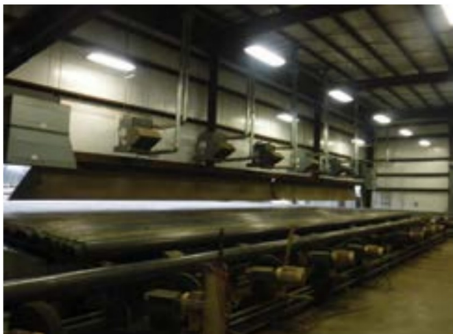
Fig. 4: View of air-heating units to warm pipes.
