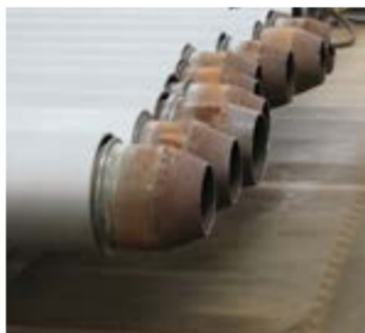
Fig. 7: Pipes after surface preparation with pipe connectors attached.
