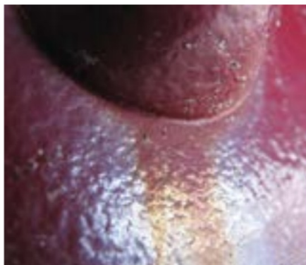
Fig. 6: Close-up of stain underneath rivet.
