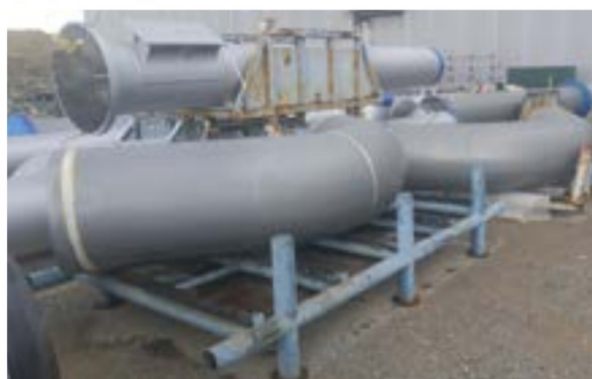
Fig. 4: Pipe spools coated with alkylated amine epoxy technology.
