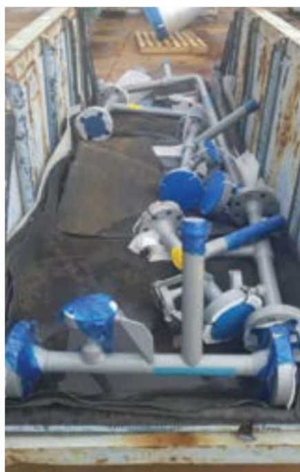
Fig. 3: Pipe spools coated with alkylated amine epoxy technology.
