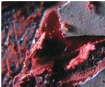
Fig. 5: Cracking pattern on topcoat and primer.
