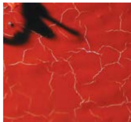
Fig. 3: Cracking pattern on primer consisting of traces of the gray topcoat.
