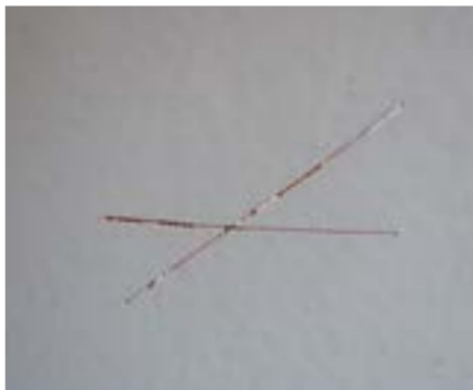
Fig. 4: Good adhesion of the coating on Lot 1 pipe.
