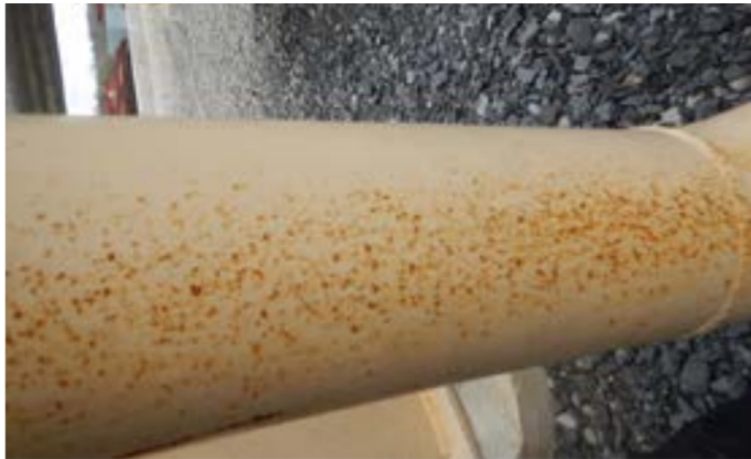
Fig. 4 (Clockwise from left): Pinpoint corrosion was observed on the piping, structural steel and flanges. Note that these surfaces were not abrasive blast-cleaned.
