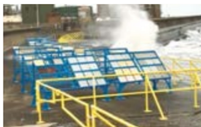
Fig. 1: Natural exposure site in the northeast of England (CX environment). Figures courtesy of the authors.
