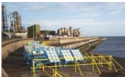
Fig. 1: Natural exposure site in the northeast of England (CX environment). Figures courtesy of the authors.
