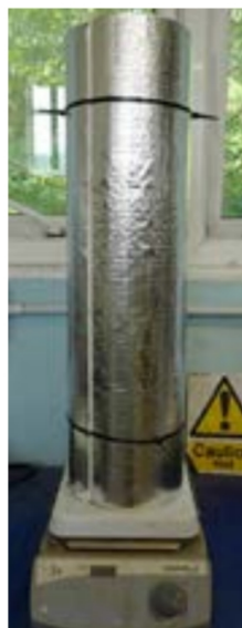
Fig. 2: Houston pipe test experimental setup for IMM-coated carbon steel pipes.
