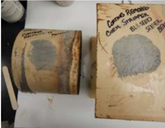
Fig. 5: Chemical stripper was used to remove coatings from shop-coated pipe and I-beam samples.
