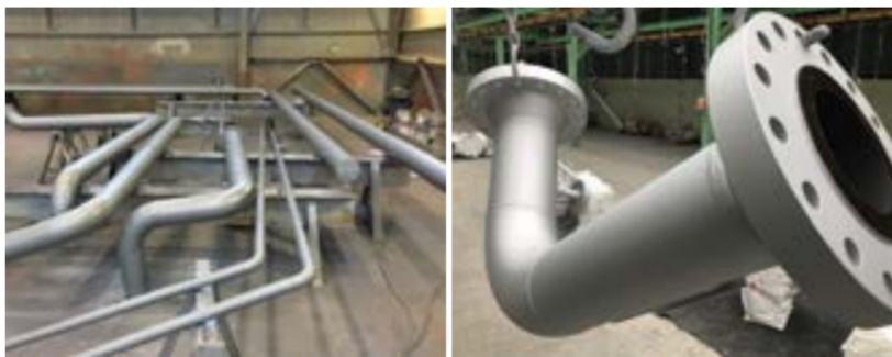
Fig. 12: Pipes and flanges coated with the novel IMM 1 coating system.
