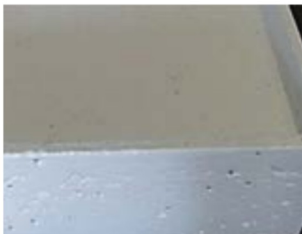
Fig. 6: Coated salt-ponding block with pinholes remaining.
