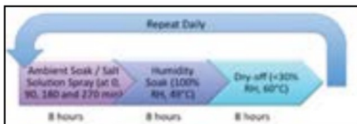
Fig. 5: One cycle of GMW 14872.
