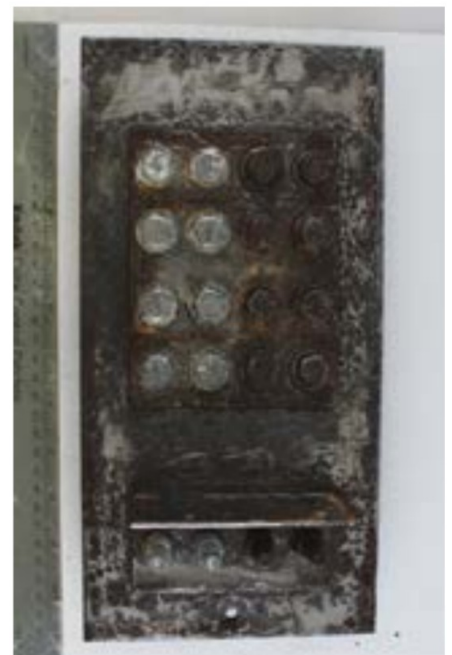
Fig. 2: Surface preparation after weathering (SSPC-SP 10 left, SSPC-SP 11 right).
