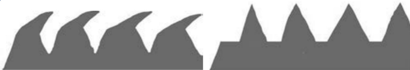
Fig. 7: Possible orientations of peaks after oblique reblasting. Rolled over peaks from reblast (left) and pushed peaks from reblast (right).
