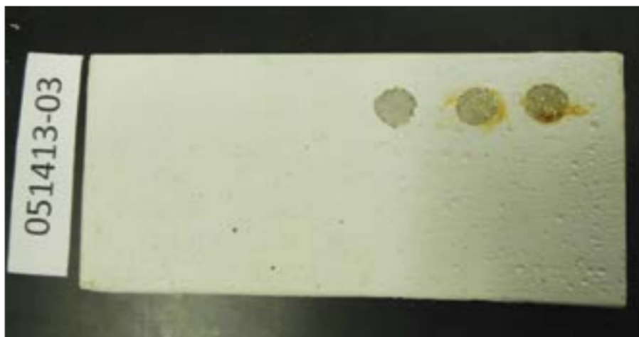
Fig. 8: Coated concrete panels for weathering testing.
