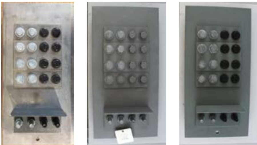
Fig. 3: New steel panels (assembled prior to blast, left; post-SSPC-SP 10 blast, center; and SSPC-SP 10 blast and primed, then assembled, right).
