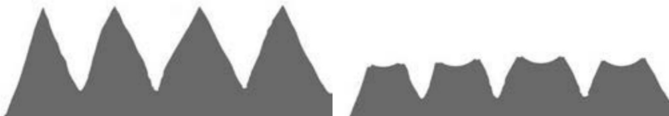
Fig. 2: Effect of reblasting a profile with a secondary blast cleaning. Original blast profile (left) and same profile after blasting with a smaller steel grit (right).
