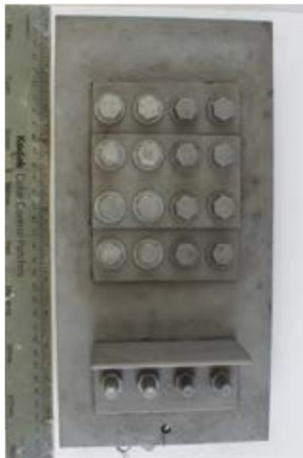
Fig. 2: Surface preparation after weathering (SSPC-SP 10 left, SSPC-SP 11 right).
