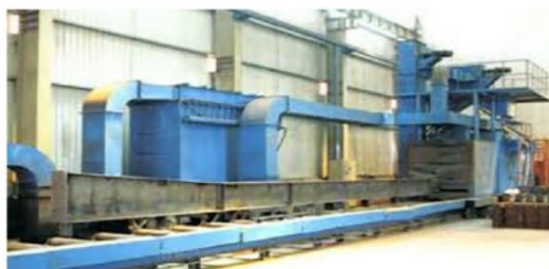
Fig. 3: Shop cleaning and painting allows for a controlled atmosphere.
