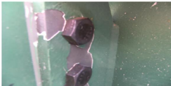
Fig. 1: Once the bolts were tightened on the surfaces which had all three coats applied, failures occurred with the intermediate and topcoats fracturing down to the primer. Figures courtesy of the author unless otherwise noted.
