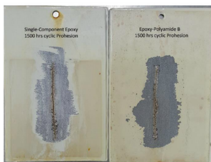
Fig. 4: 1,500 hour cyclic prohesion before stripping (above) and after stripping (below).
