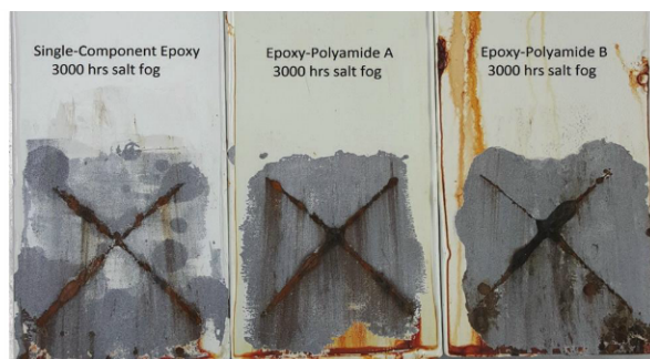
Fig. 3: 3,000 hour salt fog panels before stripping (left) and after stripping (above).
