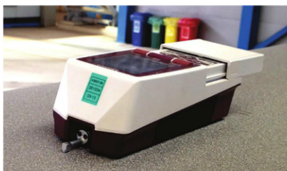
Fig. 1: For this set of tests, a profilometer measured a peak to valley height of 70-to-100 \mu\text{m} (~3–4 mil) and an average peak count of 41/cm (104/in).
