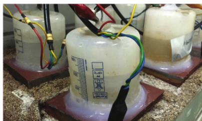
Fig. 2: Both the short- and long-term CD tests were conducted at 65 C (150 F), -3.5 V (calomel reference electrode) and a 3-percent NaCl electrolyte.
