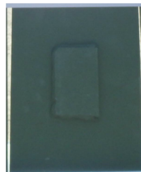
Fig. 5: Hand tool prepared panel ready for exposure in Ft. Lauderdale, Fla.
