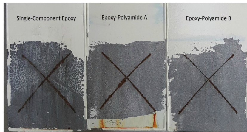
Fig. 1: 1,000 hour salt fog panels before stripping (above) and after stripping (below).
