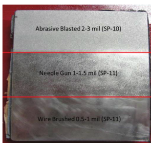
Fig. 1: This images shows the final surface profile types.
