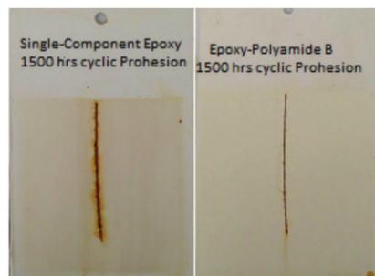
Fig. 4: 1,500 hour cyclic prohesion before stripping (above) and after stripping (below).
