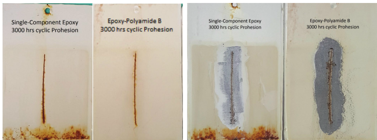
Fig. 5: 3,000 hour cyclic prohesion before stripping (left) and after stripping (right).
