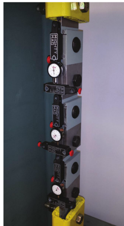
Fig. 5: Close up of a single tension creep chain. The plates are installed with coated surfaces in contact with coated surfaces and bare surfaces in contact with bare surfaces.
