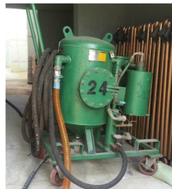
Fig. 9: A portable blasting machine was used to propel the abrasive.
