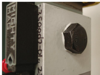
Fig. 6: Samples are assembled for tension creep to determine the effect of the full coating system applied to the backside. Note the visible compression of the coating after pretensioning the bolt.
