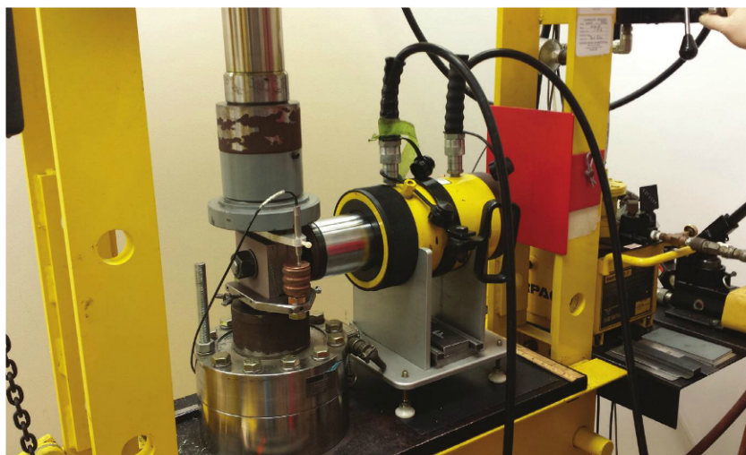
Fig. 2: Slip coefficient test apparatus with testing underway. A vertical load is applied to the center of the three plates to induce slip.
