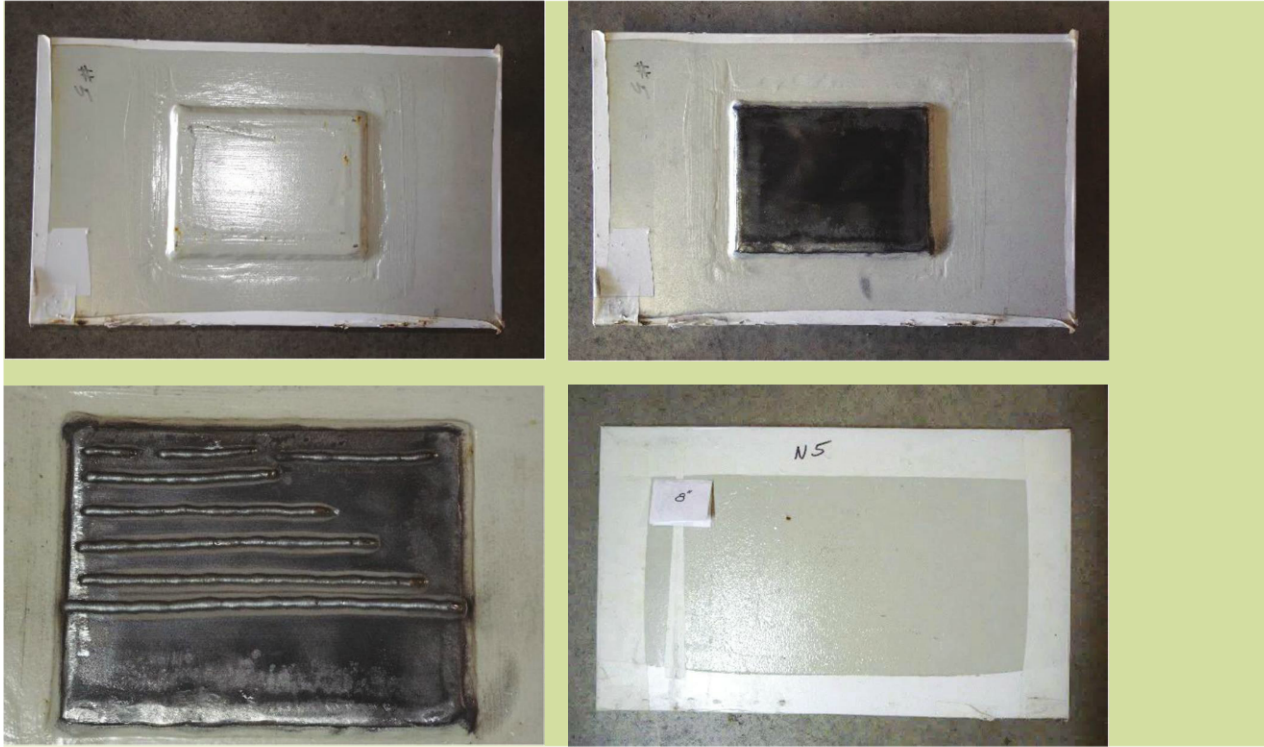
Fig. 1 (top left): The base material of the test plate used in all testing consisted of a ¼-inch-thick A36 steel plate with a ¼-inch-thick A36 steel reinforcing pad welded in place resulting in a total test plate thickness of a one-half-inch.
