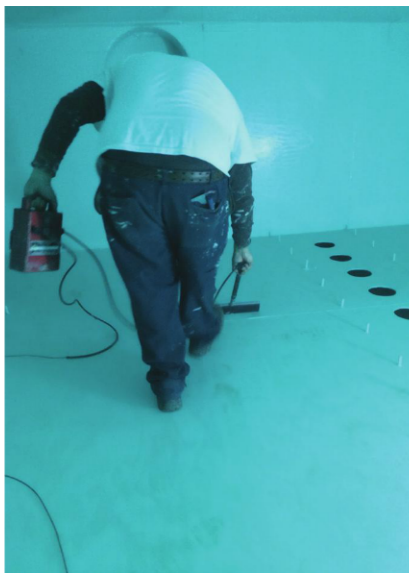
Fig. 5: Holiday testing of a 100-percent-solids epoxy coating ensuring that the coating had covered all surfaces of the steel.
