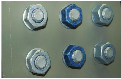
Fig. 8: The initial appearance of the lubricant/dye (center) and the appearance after cleaning for a project-specific cleaning evaluation.
