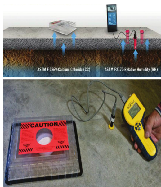
Fig. 1: These photos show the test set-up for both ASTM F1869 and ASTM F2170. All figures courtesy of the author.
