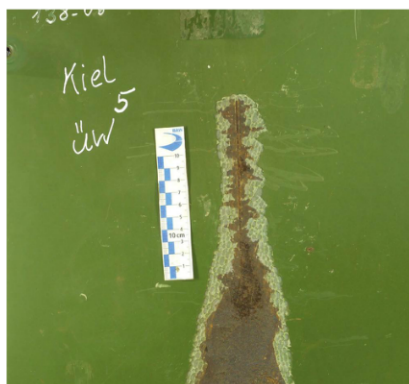
Fig. 3: Significant rusting in splash zone after five years of exposure. (Zn-free system, Norsok A.7).
