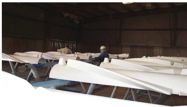
Fig. 4: An entire yard crew was trained in the special abrasive sweeping and coating application requirements of the project, and close quality control was maintained cooperatively by all the parties involved.
