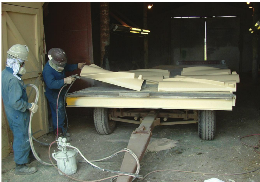
Fig. 7: After having been abrasive swept, stub riser cover pieces, too short for the pipe racks, were coated on the back of a shop trailer.
