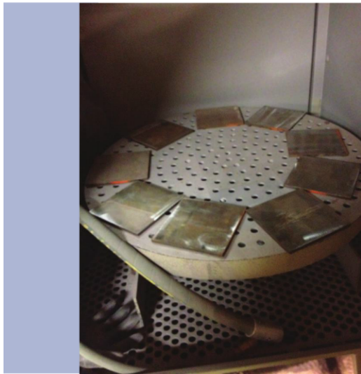
Fig. 1: Panels arranged for blasting in glove box blasting cabinet.
