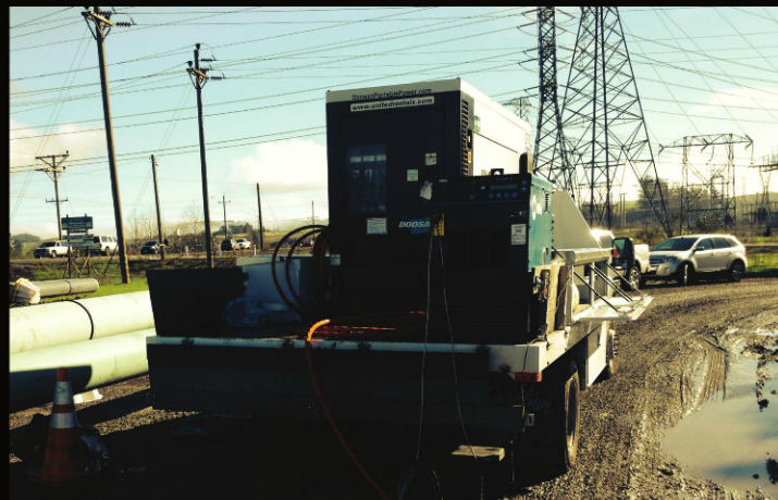
Fig. 3: Induction heating system mounted on a vehicle for use in pipeline right-of-way.
