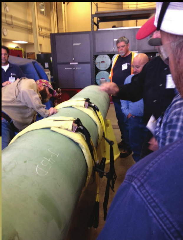
Fig. 1 (Left): Induction heating equipment set up for demonstration at PG&E Applied Technology Services facility.
