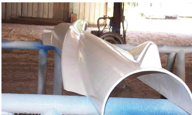
Fig. 2: As a test of effectiveness, the fiberglass fabricator prepared a single half-shell, which was then blasted and coated, to be shipped offshore for a test on an actual riser in the Gulf of Mexico.
