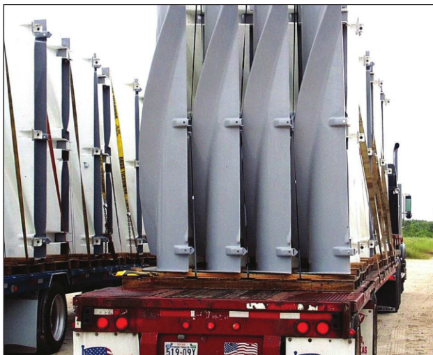
Fig. 6: Larger-diameter covers were shipped standing on edge on a flatbed truck, and were laid flat on the back deck of the supply boat to prevent damage to the applied coating.
