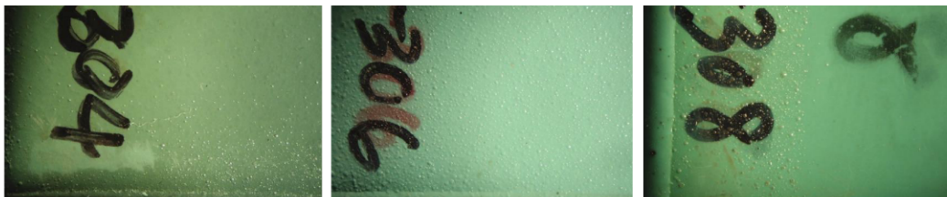
Fig. 3: Surface blisters on SFE 1 in prequalification testing.
