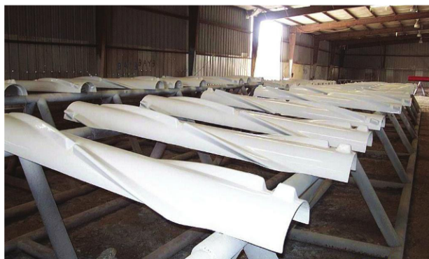
Fig. 3: What had for months been a one-off test program came to take over an entire building, as abrasive sweeping and coating of the riser cover half-shells expanded into a multi-year, multi-million-dollar assembly-line project.
