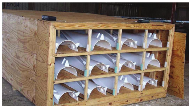
Fig. 5: Special plywood housings were fabricated for the smaller-diameter riser covers, as much to prevent damage to the NBFRS antifouling as to be sure the covers floated if they went overboard from the back deck of a supply boat.
