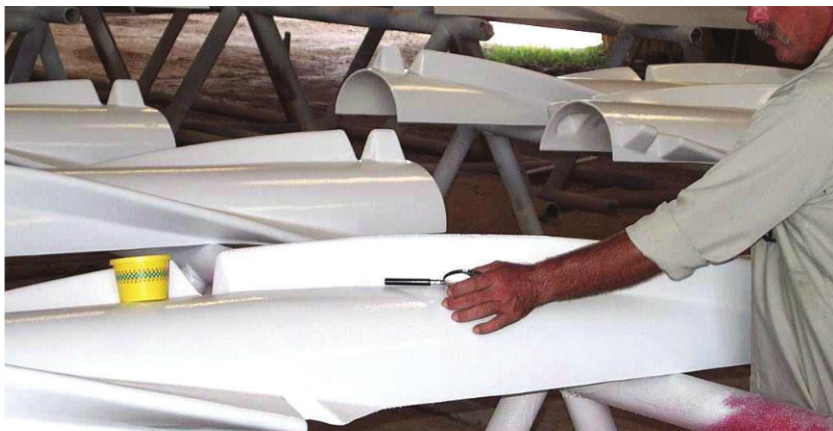
Fig. 1: Prepared surfaces of the riser covers had to be 100-percent checked with low magnification, and filling in pinholes was a process similar to final preparation of auto body panels in a body and fender shop before application of the first coat of paint.
