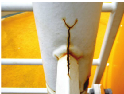
Fig. 9: Cracks in a coating film caused by inner tensions in the coating film from excessive DFT. Photo courtesy of FORCE Technology.
