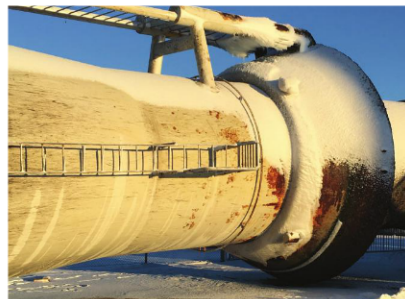
Fig. 4: This image shows a decommissioned TP from Yttre Stengrund Wind Farm, Baltic Sea, Sweden, after more than 15 years of service. The splash zone area has been attacked by ice, other impacts and general wear. The area above the splash zone is in fairly good condition. The brackish, low-saline water and the cold climate of the Baltic Sea may have contributed to the lesser corrosion. Photo courtesy of FORCE Technology.
