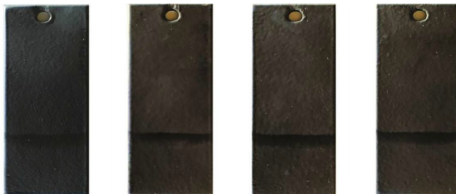
Fig. 5: Coating 2 panels, post autoclave test. (Left to right): 2A, 1B, 2B and 1C.
