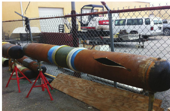
Fig. 1: View of a pipe section over pressure testing. Photos courtesy of the author unless otherwise noted.
