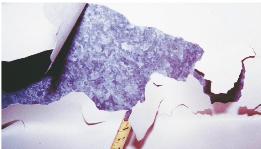
Fig. 2: Coating delamination at a galvanized surface.
