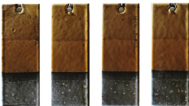
Fig. 4: Coating 1 panels, post autoclave test. (Left to right): 2A, 1B, 2B and 1C.
