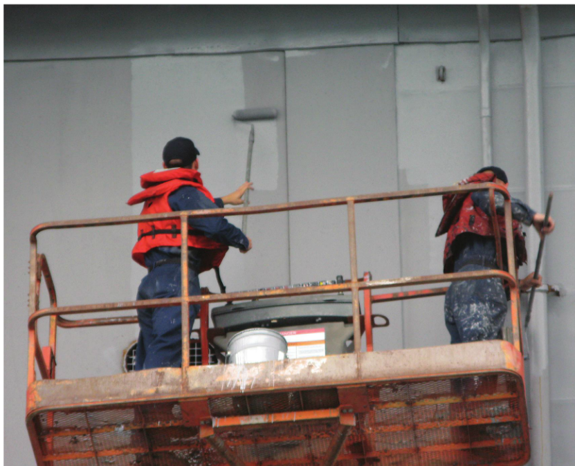
Fig. 2: Sailors roll-apply fresh silicone alkyd.
