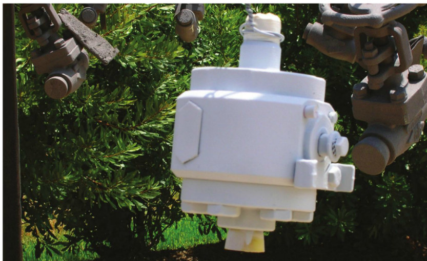
Fig. 3 (Top): Rough surface texture and a wide variation of dry film thickness readings on a small valve are the typical result of airless spray application.
