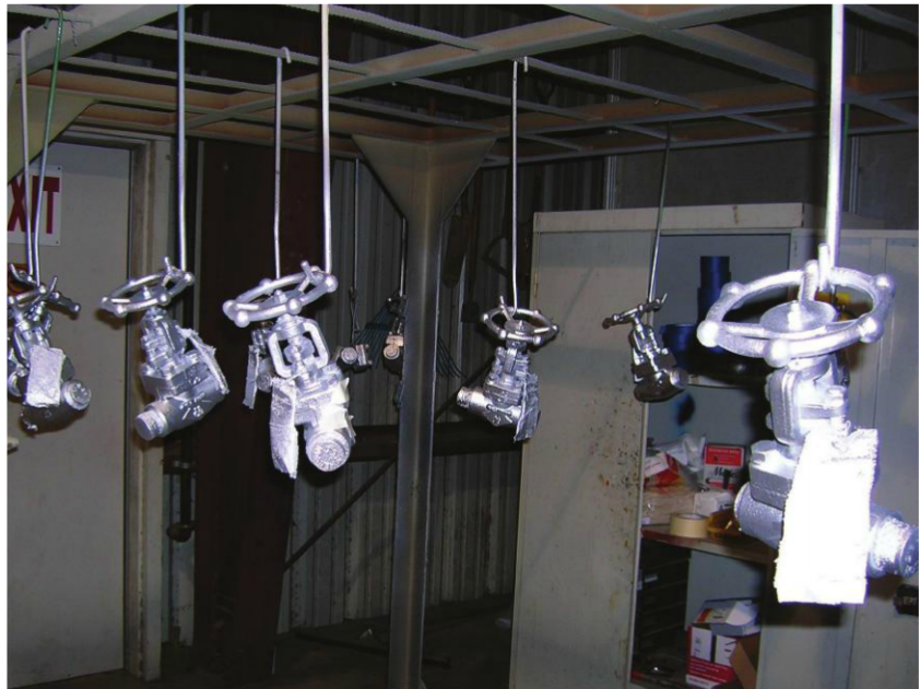
Fig. 1: Small valves with complex surfaces require conventional spray application for uniform dry film thickness and acceptable appearance. Photos courtesy of the author.
