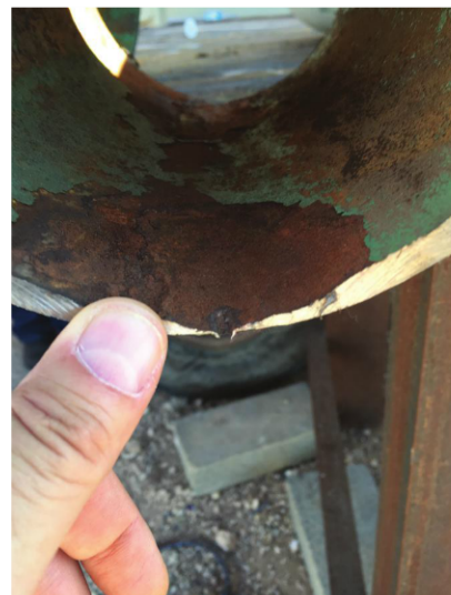
Fig. 3: Significant corrosion surrounded a perforation in the pipe.
