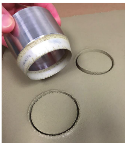
Fig. 1: DIN 18555-6 calls for the use of a tapered ring to create cuts into freshly cast mortar.
