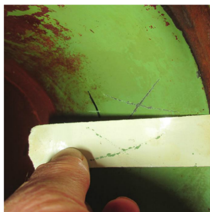
Fig. 9: X-cut adhesion testing was performed as per ASTM D3359 where the coating appeared to be reasonably well-adhered.
