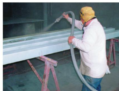
Fig. 5: Sweep blasting of galvanized steel surface.
