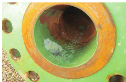
Fig. 10: Adhesion testing exposed a white coating or primer beneath the green coating.
