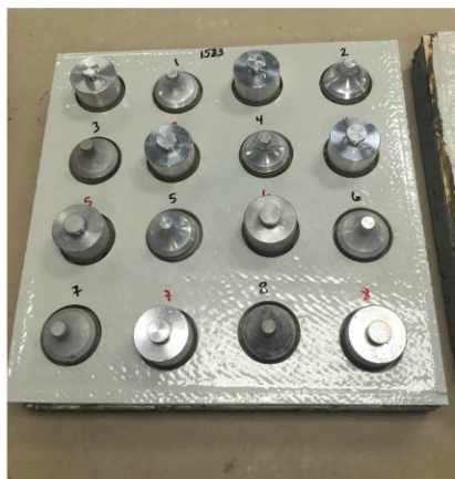
Fig. 3: A selection of 50-mm fixed and self-alignment dollies.
