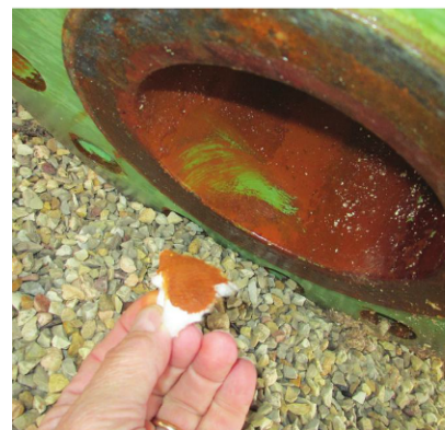
Fig. 2: A dark residue on the pipe interiors was sometimes easy to remove and sometimes difficult to remove, even with solvent.
