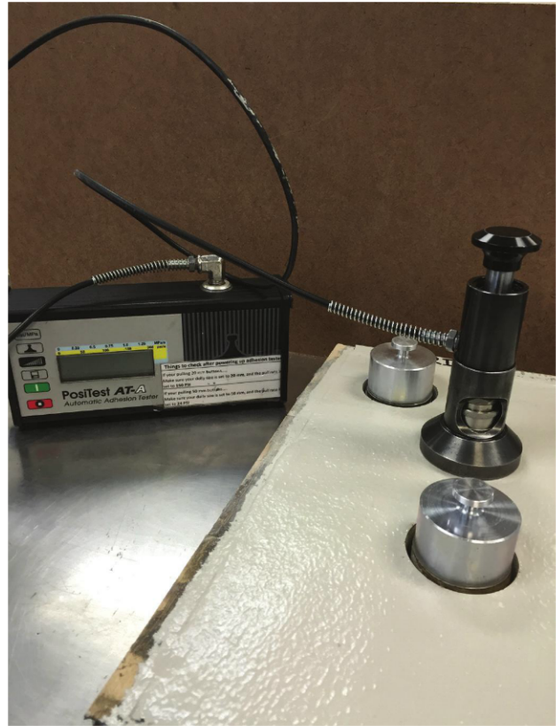
Fig. 5: A self-alignment adhesion tester.
