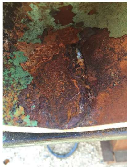
Fig. 7: An area of poorly applied coating with severe corrosion and undercutting.
