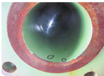
Fig. 4: Holidays were found in an area of pipe interior where the coating was otherwise intact.
