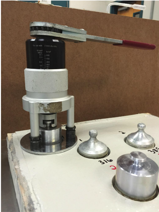
Fig. 4: A fixed-alignment adhesion tester.
