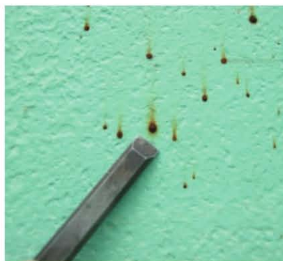
Fig. 2: Pinpoint corrosion nodules that formed on the coated carbon steel. Photo courtesy of the authors.
