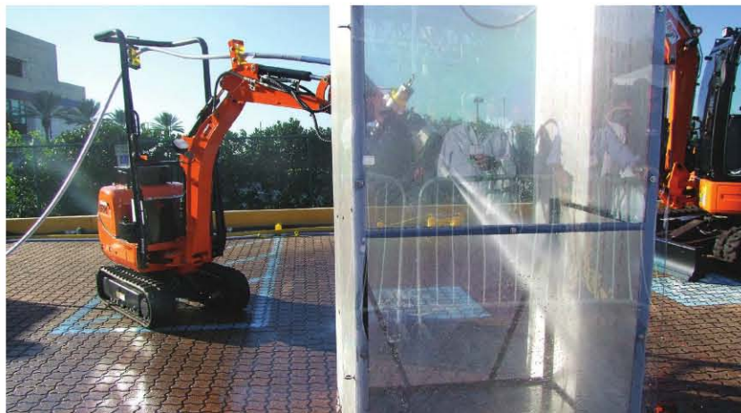
Fig. 2: Mobile robotic waterjet tools controlled by an operator at a distance.
