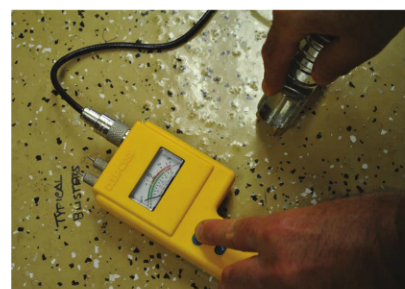
Fig. 2: Moisture tests being conducted with a moisture meter based on electrical resistivity.
