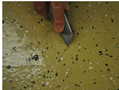
Fig. 5: Knife adhesion testing (ASTM D6677).
