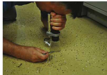
Fig. 6: Field microscopic examination of a failing area.
