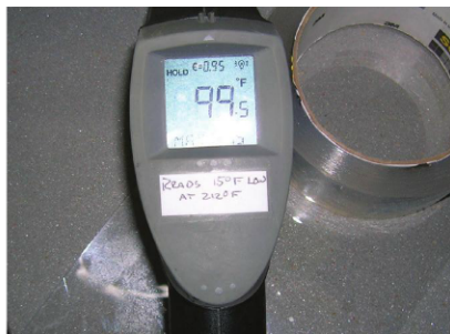
Another balmy day inside Tank 2003 — 99.5 F and about 40 percent relative humidity assured proper curing of the applied vinyl ester, regardless of weather conditions outside the tank.
