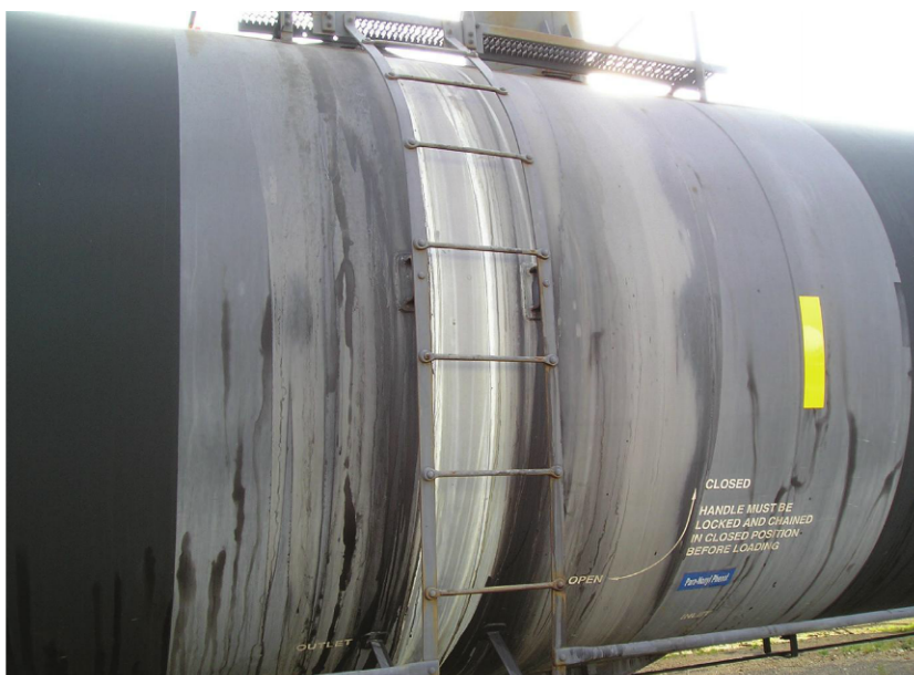
Fig. 1: The "centerband" area of a railcar is where loading and unloading operations are performed and is susceptible to spillage. Exterior coatings can be damaged if corrosive materials are involved.
