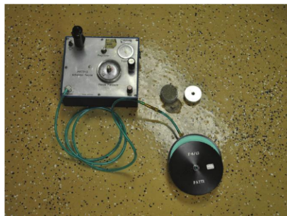
Fig. 4: Pull-off adhesion testing using a hydraulic adhesion tester (ASTM D7234).
