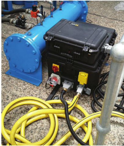
Each robot is controlled by a portable safety controller and rugged computer, shown here installed next to the blast pot.
