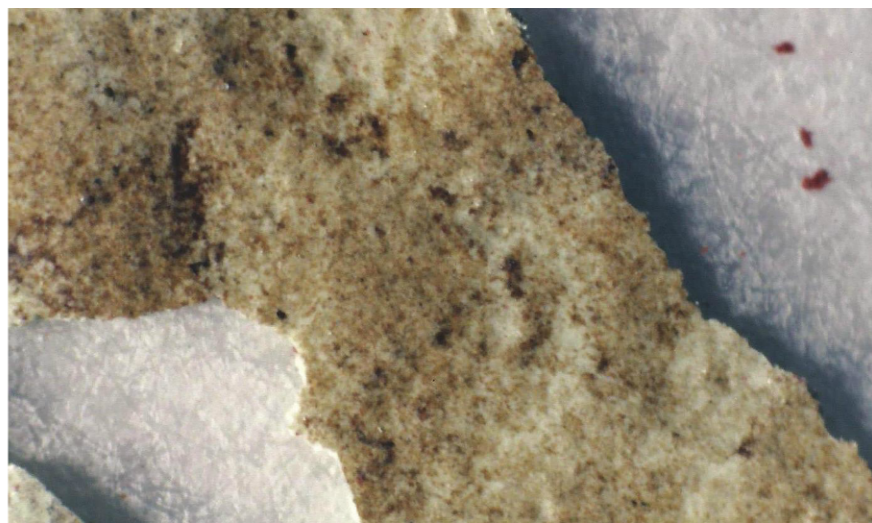
Fig. 2: Dirt on the backside of poorly adherent topcoat.
