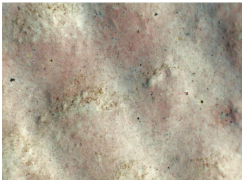
Fig. 3: Reddish residue of chalked primer on the back of poorly adherent topcoat.
