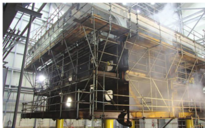
FPSO P66 being assembled (top), block being UHP waterjetted inside blasting chamber (above) and surface-tolerant coating being applied (right).
