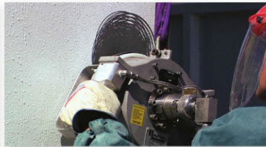
Hand-held VertaJet™ Lightweight, with vacuum recovery
