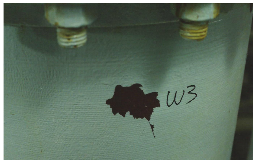
Fig. 1: Adhesion test taken at a good location, showing that poor adhesion was much more widespread than initially thought.
