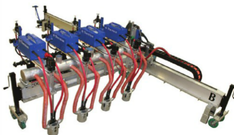
4 Head RDM-4 Robot with Direct Head Fume extraction
