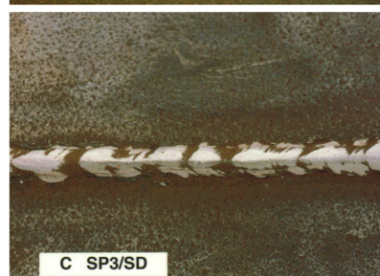
Fig. 2: SSPC visual standards for hand- and power-tool cleaning for original rust grade C. Photos courtesy of SSPC.
