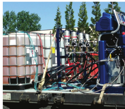
Fig. 3: Bridge deck membrane equipment setup. Photos courtesy of Dudley Primeaux.
