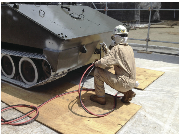
(Above photos) Reggie Clements of Vulcan Painters, Inc. sprays the M114 Command and Reconnaissance Carrier.
