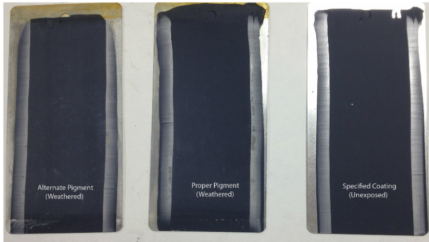
Fig. 2: Variances in pigmentation led to differences in performance and aesthetic properties for this specified coating in Case Study 1.
