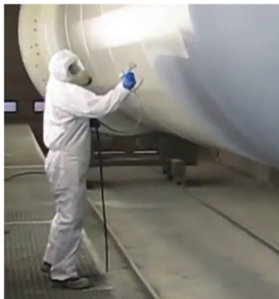
Workers applying plural-component spray coating to pipe exterior. Photos courtesy of WIWA LP
