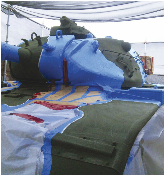
Masking the camo pattern on the M60A3 (left). Below, the M3 Bradley fighting vehicle before painting. Zachary Daniels and Hyrum Zweifel of Coatings Unlimited, Inc. apply the finish coat to the primed Bradley (bottom).
