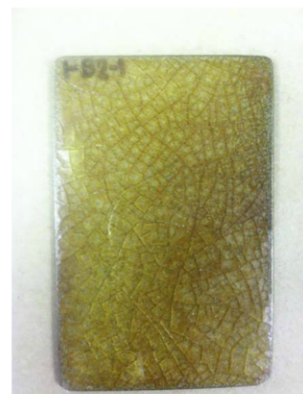
Fig. 2: Novolac epoxy coating exposed for short duration at 350 to 400 F.
