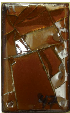
Fig. 3: Bis-A epoxy/cycloaliphatic amine with benzyl alcohol exposed to 500 F.
