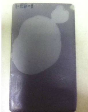
Fig. 1: Epoxy coating exposed for short duration at 350 to 400 F.
