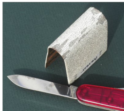
Fig. 3: This coupon failed the thermal-spray bend test after testing as specified in SSPC-CS 23.00/AWS C2.23M/NACE No. 12.
