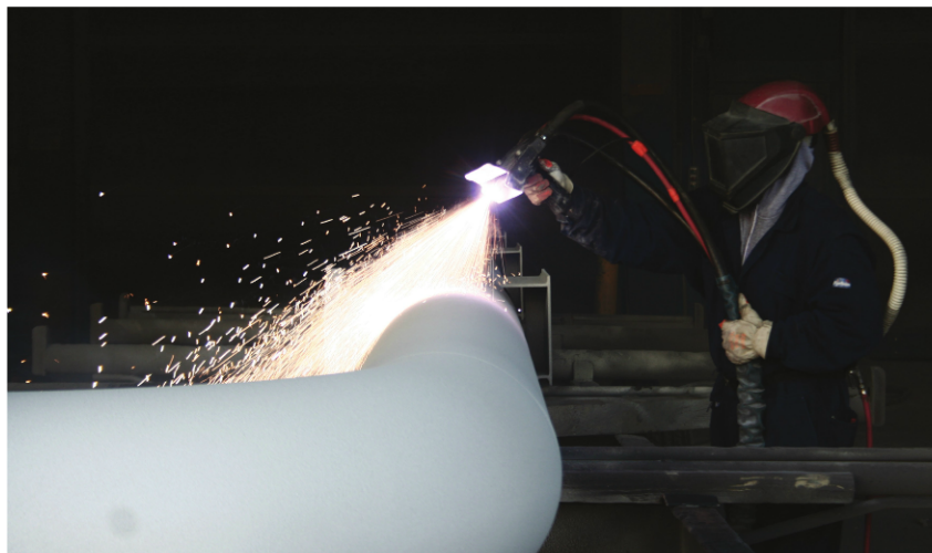
Fig 4: Despite the apparent fireworks, the arc-sprayed thermal-spray aluminum is dry and cool almost immediately after application and is ready for insulation and jacketing. Liquid coatings require additional coats and extended drying time after each coat. Photo courtesy of Turner Industries Group, LLC.
