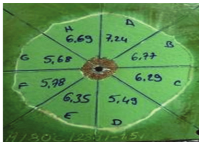
Fig. 2: Disbondment radii measurements for a sample were made along each of the eight cuts. The results are averaged and reported.
