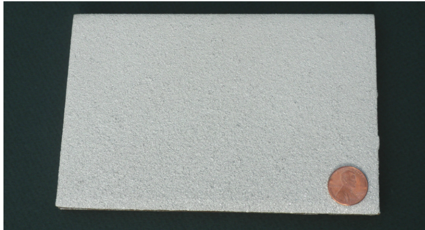
Fig. 5: Inspection of thermal-spray aluminum requires special care because the visual appearance of thermal spray is almost identical to the appearance of newly blasted steel.
