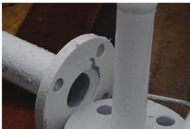
Figs. 3 and 4: Onshore-coated items, structures and piping should be better protected during shipping to minimize damage to the coating system.
