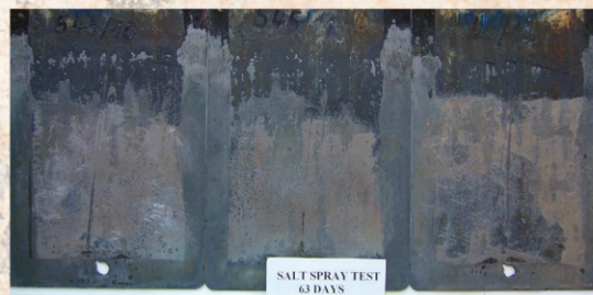
Fig. 4: High level of red rust with formulation containing 10-percent FPA (ZnF-2).
