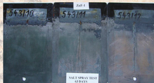
Fig. 3: Virtually no red rust with formulation containing only zinc dust (ZnF-1).
