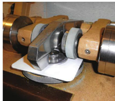
Fig. 1: This image shows a test panel mounted onto a Taber abrader, with the two abrading wheels, the weights (in this case, a 1,000-gram load) and a vacuum nozzle to remove fragments of paint as they are generated. Figures courtesy of the author.
