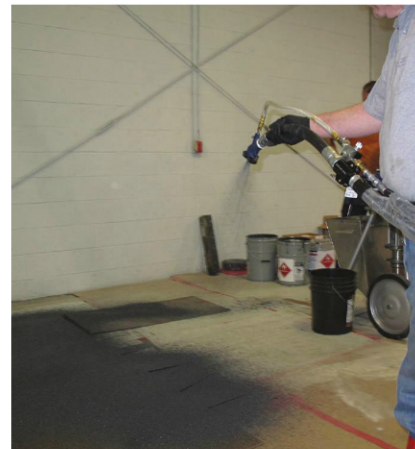
Fig. 4: During the test, a surface area of 32-square feet was sprayed in 3.9 seconds.
