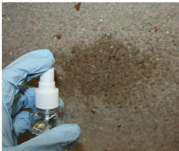
Fig. 2: This image illustrates the water drop test being performed with water flowing (wetting) the concrete surface.
