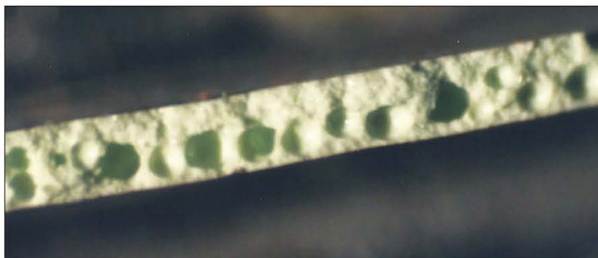
Fig. 2: This urethane shows poor adhesion to an underlying epoxy primer. Microscopic observations show a layer of voids near the back surface, indicating that the coating may have been applied over moisture.
