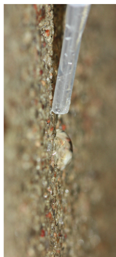
Fig. 3: A water bead forms on a contaminated surface.
