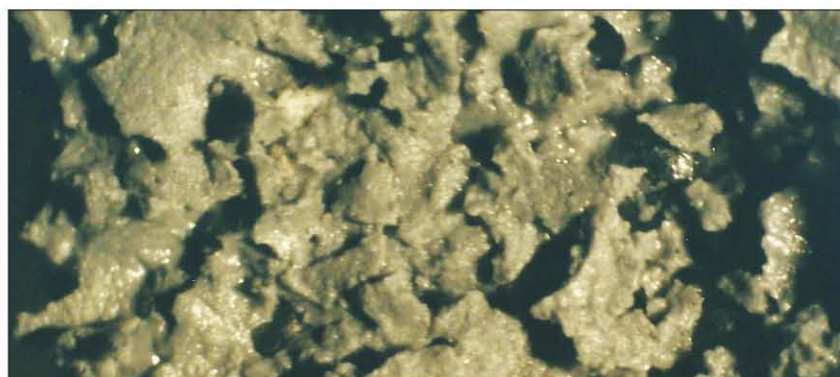
Fig. 5: This is the same chip of epoxy as shown in Figure 4 after a few drops of MEK were applied. The chip quickly became soft and gummy, suggesting that it had been applied at the wrong mix ratio.
