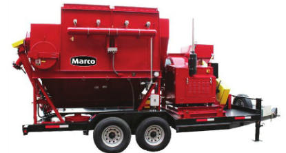
Marco's Dustmaster 8,000 CFM (top) and Dustmaster 18,000 CFM dust collectors. Photos courtesy of Marco.
