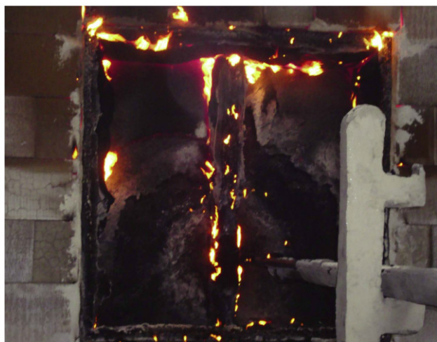
Fig. 3: These images show the progression of a typical jet fire test using ISO 22899-1.
