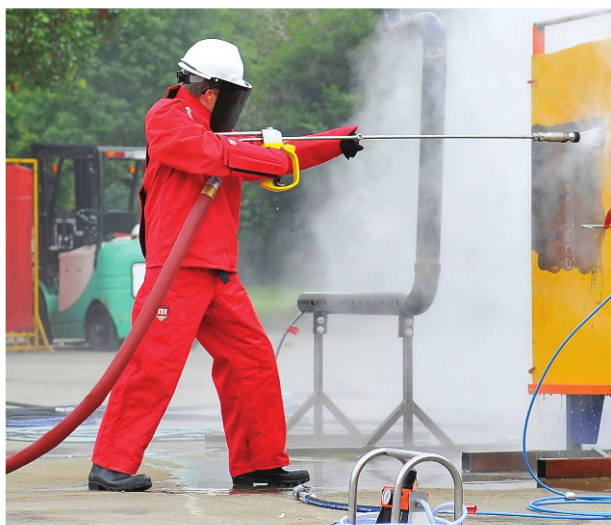
Fig. 1: Personal protective equipment, including head, eye, body, foot, hand, hearing and respiratory protection, should be worn at all times when during UHP waterjetting operations.
