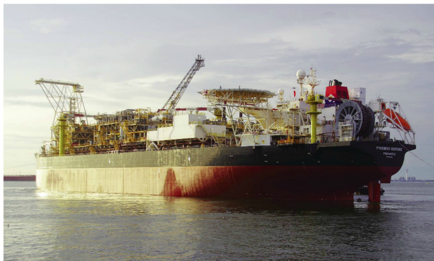
The tank deck of the donor tanker might have to be strengthened underneath the deck plates (i.e., inside the crude oil tanks) before the heavy multi-level process decks are added on top. It is quite common that the process equipment for the various parts of the production operation — including separator vessels, knockout drums, chemical dosing stations, compressors, gas turbine generators, etc., as well as workshops, cranes, the flare tower, helipad and so on — are fabricated and finished (including painting) as modules which are then sub-assembled or consolidated, craned into place and welded or affixed to the hull.
