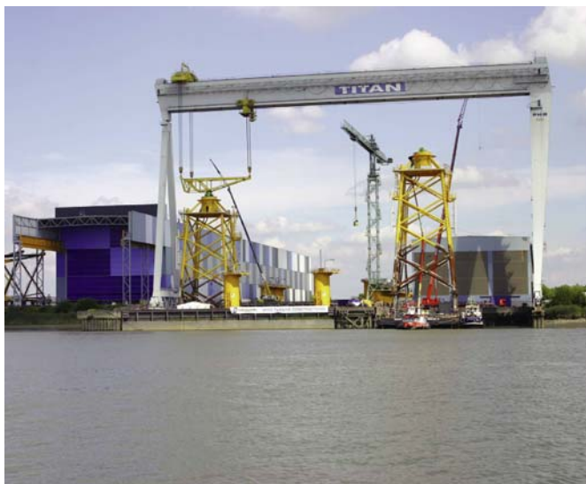
(Above and below): Finished jackets were loaded from the facility onto barges and then shipped out for placement at the Thornton Bank.
