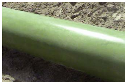
Fig. 6: Inspection of rigid test coating after 15 months. No defects or damages were observed.
