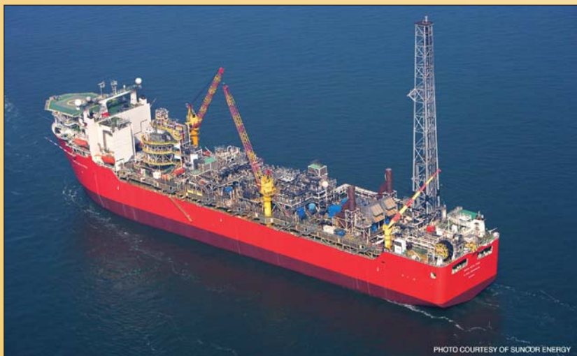
Suncor Energy uses HoldTight®102 to remove salts from its FPSO Terra Nova and other similar vessels in the North Atlantic every time it re-coats decks, structural steel, piping and other surfaces exposed to the sea.
