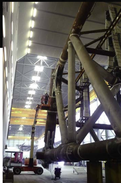
(Top of page and above): Individual steel members are brought to one of the contractor's large blast and paint facilities, where they are welded together, blasted and coated.
