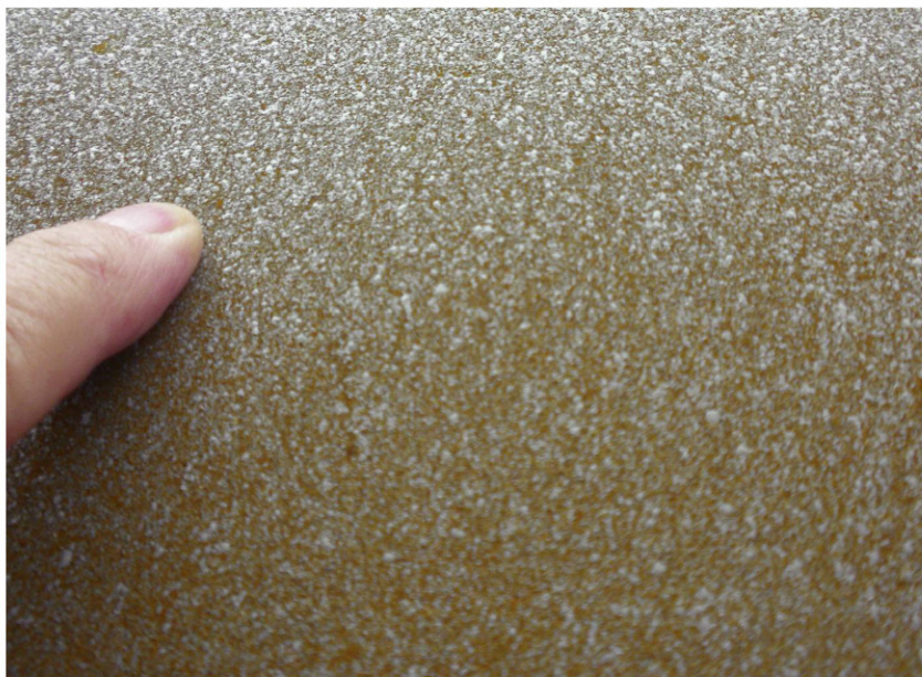
Light flash rusting on steel dry blasted to SSPC-SP 10. This area needs to be reblasted.
