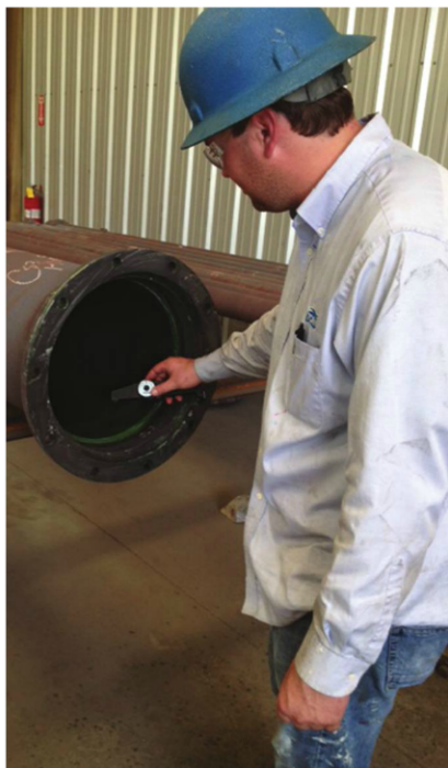
Post-application inspection procedures, including dry film thickness testing, are usually included in painting specifications. Photo courtesy of Vulcan Painters, Inc.
