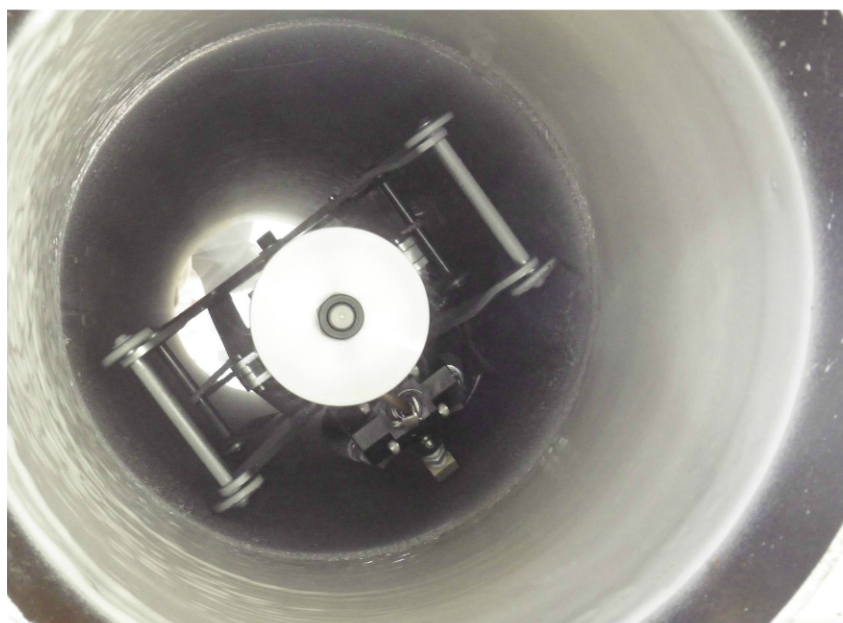
Fig. 2: High revolution-per-minute spinning cup
