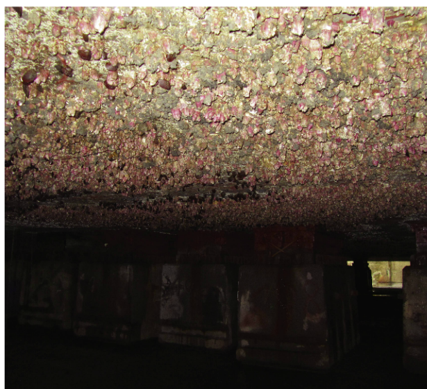
Severe marine fouling causes drag and excess fuel usage.
