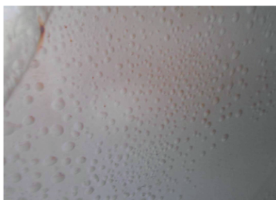
Fig. 1: Dense osmotic blistering. All figures courtesy of KTA-Tator, Inc.
