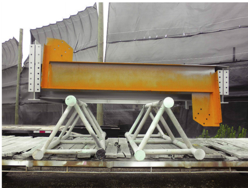
Newly-blasted support beam unit has flash rusted badly after an unexpected rain shower.
