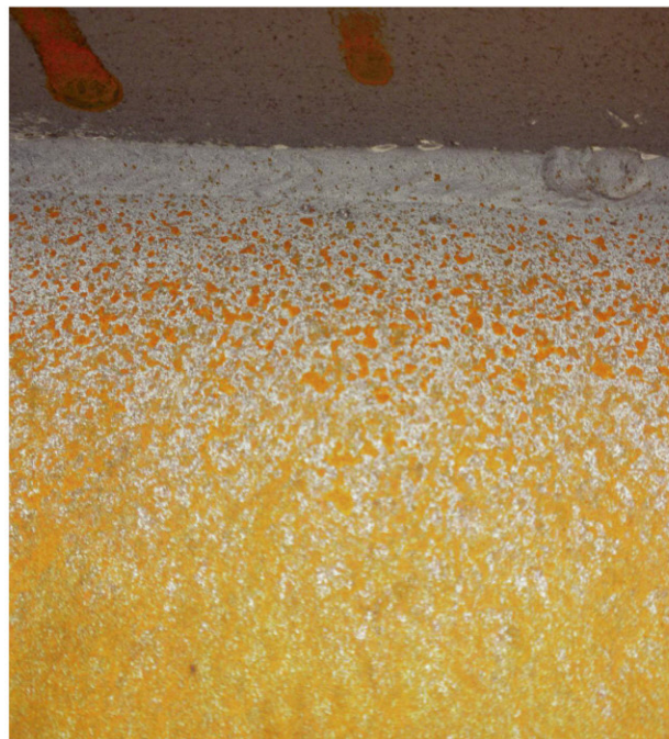
Moderate flash rusting on steel dry blasted to SSPC-SP 10.
