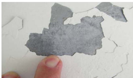
Fig. 5: The galvanized metal substrate is visible after the loosened Coating B was removed. Apart from a slight waxy feel, the saponified layer is transparent and must be confirmed by analytical testing using IR analysis.
