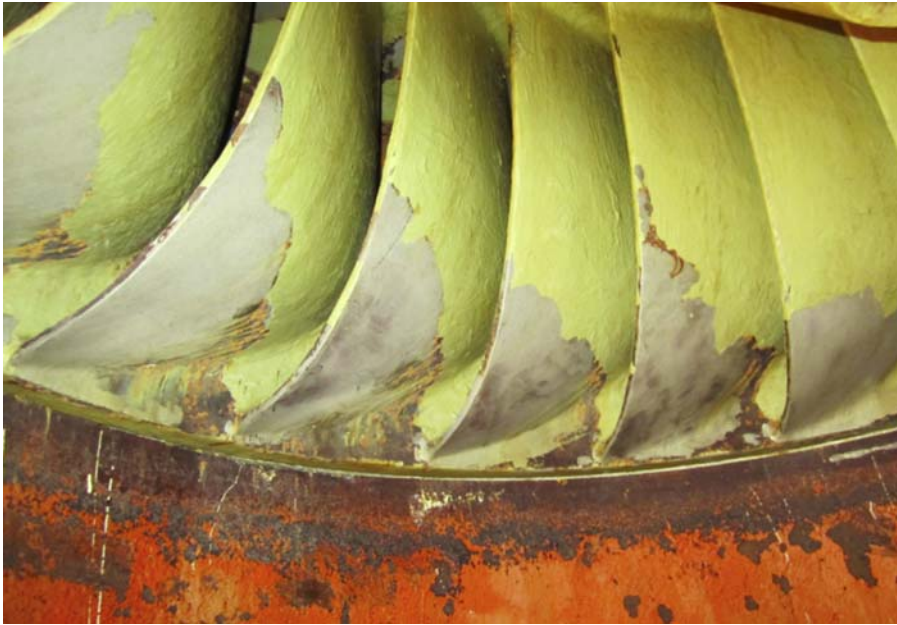
Fig. 6: Turbine runner and draft tube with coating and cavitation damage
