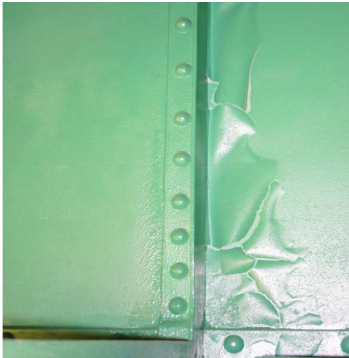
Figs. 4 and 5: Coating System J, the elastomeric acrylic, showed blistering, peeling and corrosion on approximately 20 percent of the total surface area.
