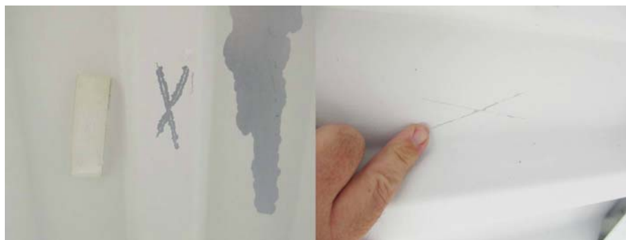
Fig. 4: Photo at left depicts adhesion test result on surface with Coating B. Photo at right depicts test result of surface with Coating A.
