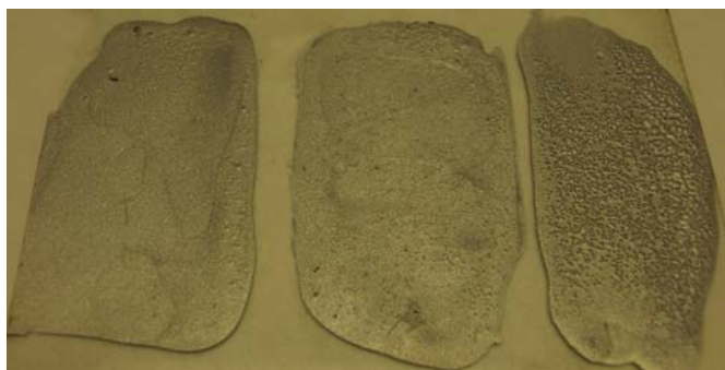
Fig. 2: Over-catalyzed material formed bubbles, creating an uneven surface. Foaming occurred at the incorrect mixing ratio on the right side.
