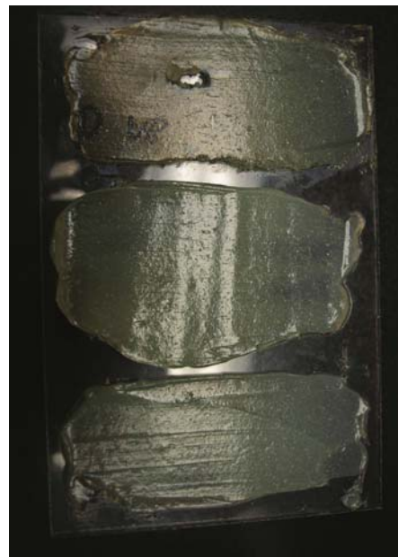
Fig. 5: Three mixes that were similar in gloss and appearance displayed variations in hardness.
