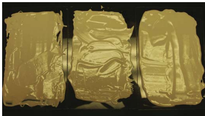
Fig. 1: Three mixes of the same material all cured to glossy finishes with the same hardness. Photos courtesy of KTA-Tator, Inc.
