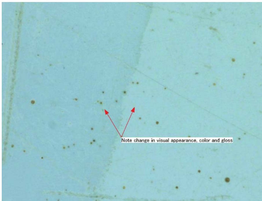
Fig. 6: Decreased abrasion resistance of an epoxy floor coating due to off-ratio mix, viewed at 50x.
